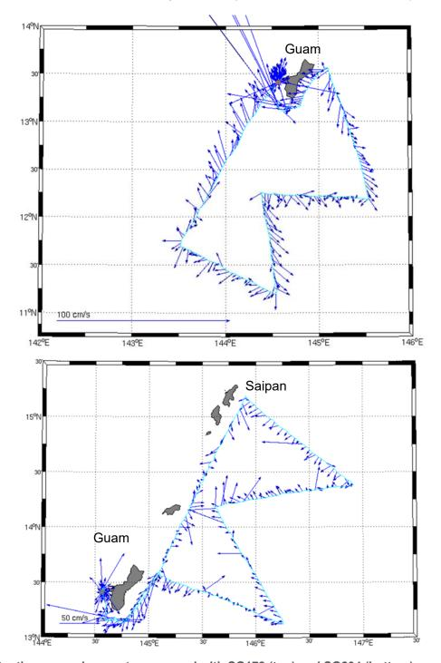
Figure 8: Depth-averaged currents measured with SG178 (top) and SG204 (bottom).
