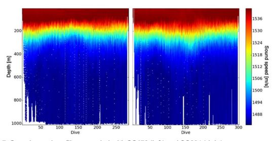
Figure 7: Sound-speed profiles recorded with SG178 (left) and SG204 (right).
