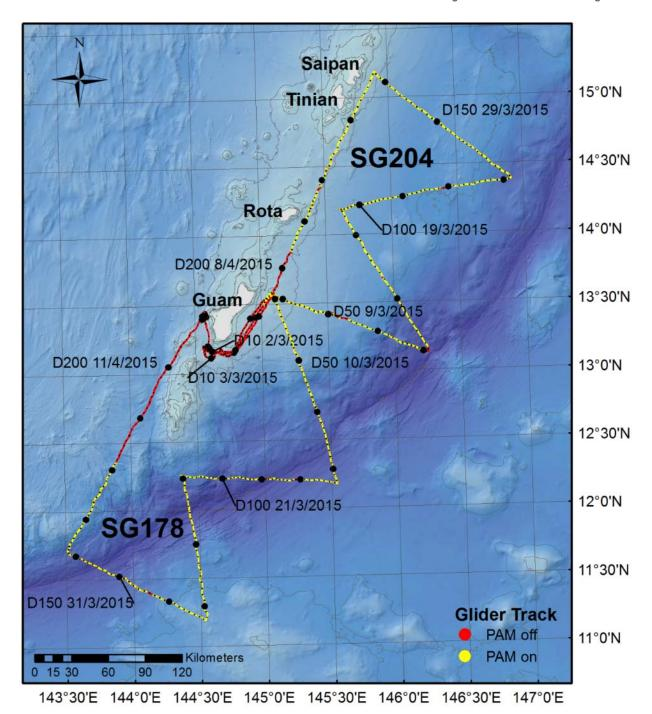
Figure 5: SG178 (south) and SG204 (north) track lines for the period 2 March to 27 April 2015. Each black dot (with every tenth one larger) on the track line indicates the midpoint location of a glider dive. Labels indicate dive number (e.g., D10 for dive no. 10) and date (format: dd/mm/yy UTC). Red sections indicate that the PAM system was switched off. The yellow segments indicate that the PAM system was active.
