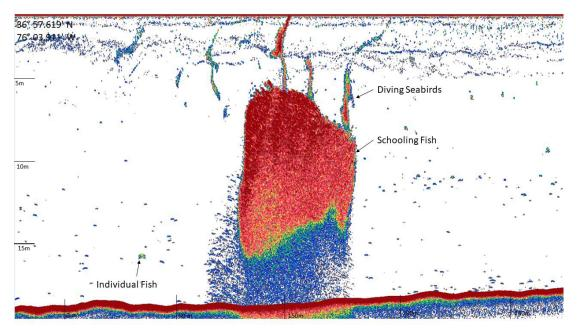
Figure 8. Example echogram showing a large fish school in the water column.
