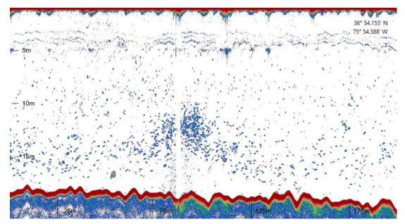
Figure 7. Example echogram showing individual scattered fish. Red color represents strong echo returns and blue represents weak echo returns.
