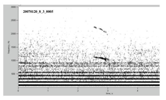
Figure 5-3. Example of Type 1A sei whale call spectrographic display showing frequency (Hz) along the y-axis and time (sec) along the x-axis with amplitude reflected as color intensity. The dark horizontal banding pattern is due to electrical noise from the research vessel's power supply. This noise only occurred during the beginning of the first leg, when, unfortunately, most of the recordings of sei whale calls were made.
