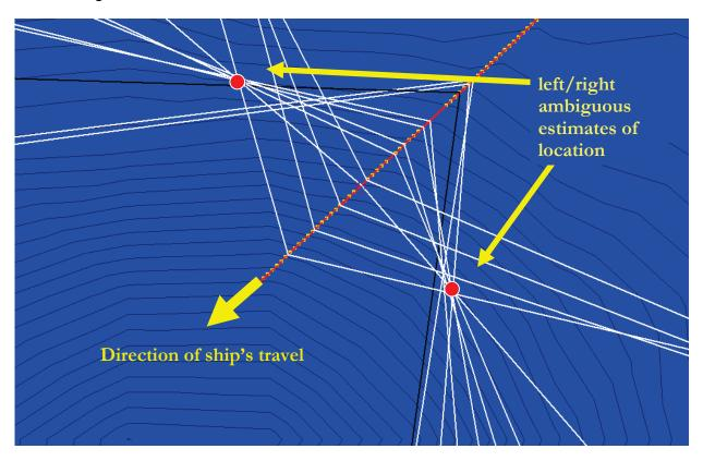
Figure 1-1. An example of the 'target motion analysis' method of localization used for minke whales. Sequential bearing lines from the towed hydrophone array to a vocalizing animal converge as the vessel passes the animal. This method assumes that the animal is relatively stationary compared to the vessel speed. Also note the left/right ambiguity caused by the linear configuration of the hydrophone array.
