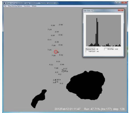
Figure 2: Custom display showing the hydrophone locations on the range with a single dive detected on phone 193 indicated by small red circle. Clicking on the phone with the detections pops up an ICI histogram (insert) for that phones automatic detections (peak IDI for this case of 0.3s). Data is from 12 Feb 2012 at 01:11 GMT.
