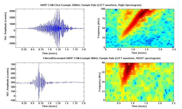
Figure 5 – Upper plots are a sample waveform and spectrogram of a Cross Seamount frequency modulated click as collected by HARP (courtesy of McDonald and Hildebrand). Lower plots show apparent reduced duration and bandwidth when filtered/decimated to simulate reception on PMRF hydrophones. Note the spectrogram axes are different – top goes to 100 kHz while bottom goes to 48 kHz.
