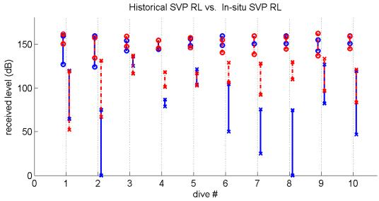
Figure 8: Estimated max/min RLs using historic versus *in situ* sound velocity profiles at 10 m and 1 km depth for each dive from Table 5. At 10 m depth: red circles are RLs from Historic SVP, blue circles are RLs from In-Situ SVPs. At 1 km depth: red x's are RLs from Historic SVP, blue x's are RLs from In-Situ SVPs.
