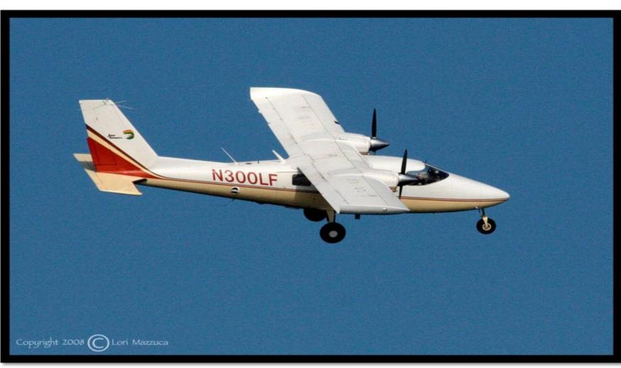
Figure 1. Partenavia twin-engine aircraft flown for aerial surveys. Line-transects were flown at 1000 ft altitude; focal observations were flown in circles from 1200-1500 ft. altitude and 0.5-1 km radial distance (outside the sound cone of plane) to avoid disturbance of marine mammals
