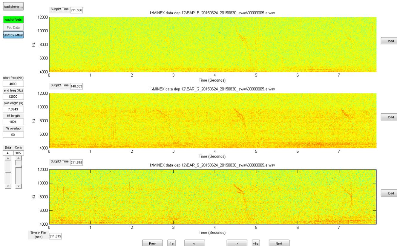
**Figure 8. Time-aligned spectrograms from three EARs in file 3005, following an explosion detected in file 3004 6 minutes earlier. Note the low SNR of the whistles at 0.5 second and 2.7 seconds on EARs B (top panel) and S (bottom panel).**
