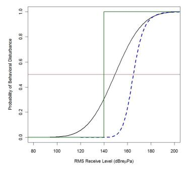
Figure 2. A comparison of risk functions relating the probability of disturbance (cessation of foraging using echolocation) to received level for beaked whales exposed to sonar signals. The current step function used by the U.S. Navy is shown by a green line and the historical function by a blue-dashed line. The empirical function developed in this paper is shown by a solid black line. A solid red line marks the 0.5 probability of disturbance.
