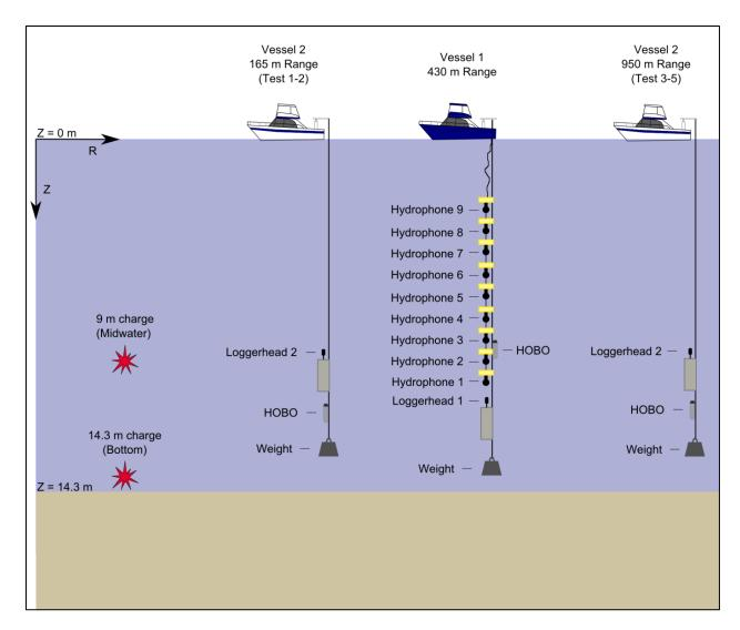
Figure 15. Experiment geometry for the Virginia Beach MINEX trial. Hydrophone depths located in
