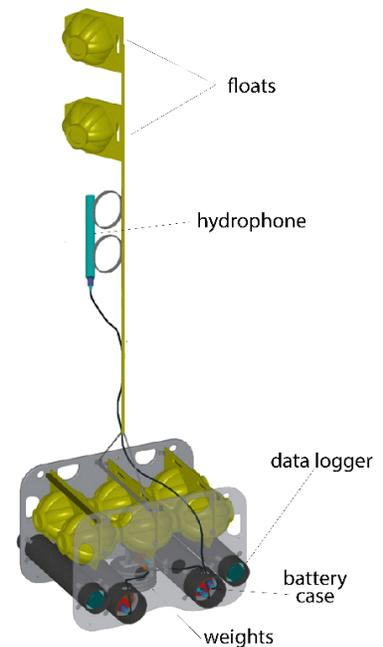
Figure 4. Schematic of a HARP seafloor package
