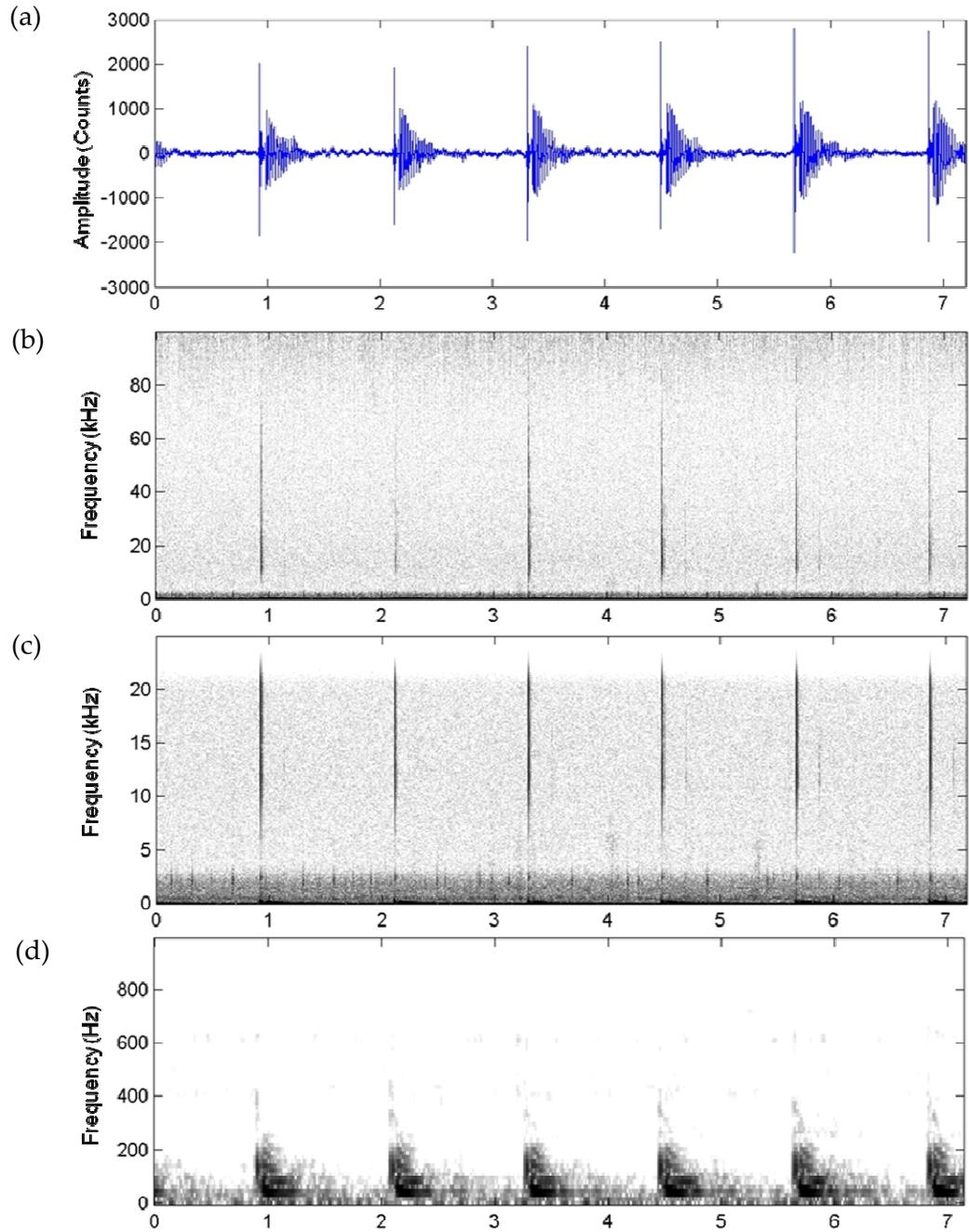
**Figure 39: Example of part of a consistent pulse train showing higher-frequency components. (a) Waveform, (b) spectrogram showing non-decimated data (sampling rate 200 kHz, FFT size 1024 samples, 75% overlap, Hann window), (c) spectrogram showing decimated data (sampling rate 50 kHz, FFT size 1024 samples, 75% overlap, Hann window), and (d) spectrogram showing decimated data (sampling rate 2 kHz, FFT size 128 samples, 75% overlap, Hann window).**
