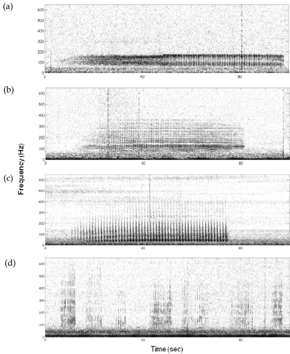
**Figure 37: Spectrograms of different types of pulse trains showing (a) slow-down, (b) speed-up, (c) consistent, and (d) short pulse trains (FFT size 512 samples, 75% overlap, Hann window).**
