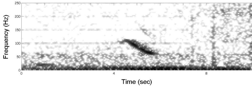
**Figure 32: Spectrogram of “hooked” downsweep (FFT size 512 samples, 75% overlap, Hann window).**
