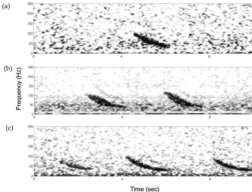
**Figure 30: Spectrograms of downsweeps occurring as a (a) single, (b) pair, and (c) triplet (FFT size 512 samples, 75% overlap, Hann window).**
