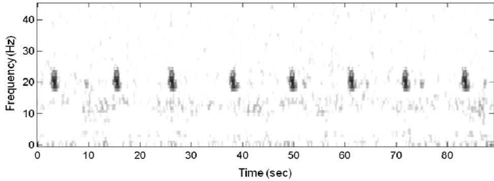
Figure 28: Spectrogram of eight 20-Hz pulses (FFT size 2048 samples, 90% overlap, Hann window).
