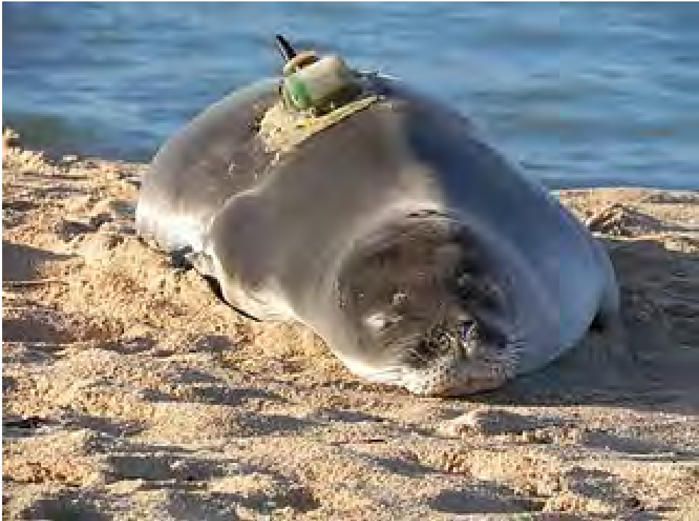
Figure 1. Photo of R4DF with a cell phone tag attached. The instrument is attached to a neoprene base, which is glued to the pelage of the seal.
