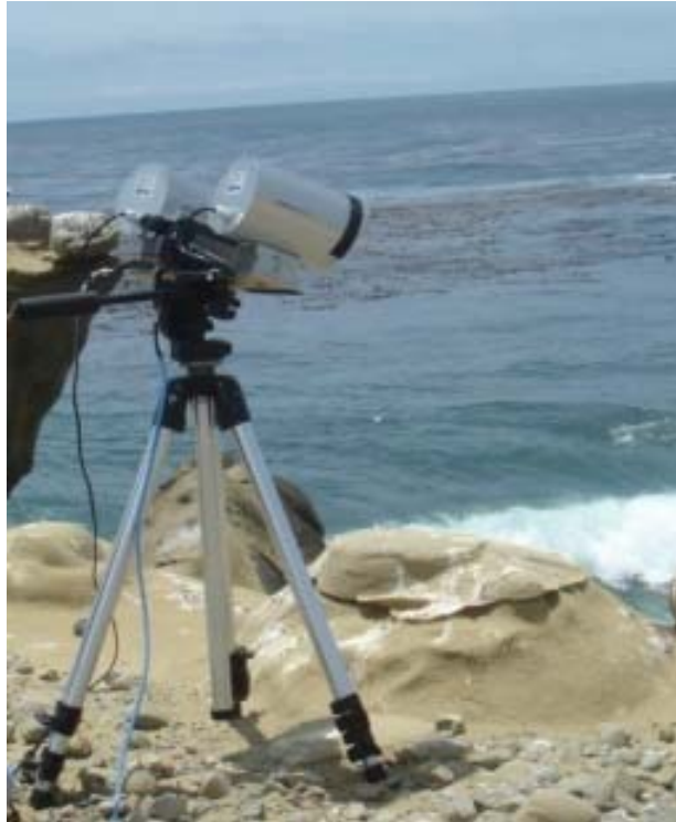
FIGURE 3.2. Photo of video camera set-up at SNI with two infrared illuminators (photograph by G. Smith, U.S. Navy).
