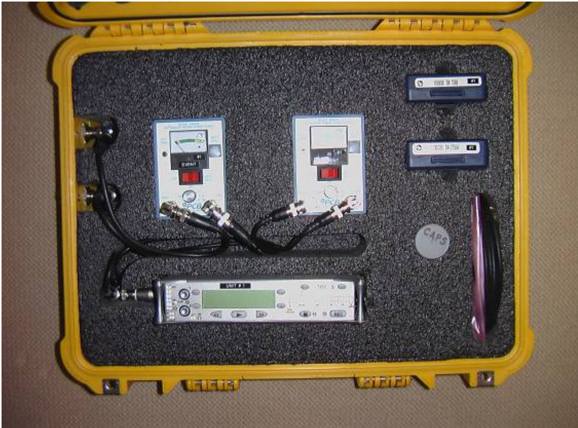
FIGURE 2.2. Photo of ATAR components in waterproof Pelican case (photograph by R. Norman, Greeneridge).
