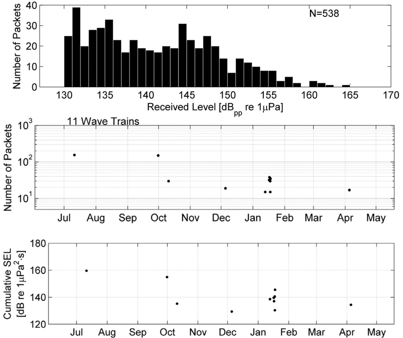
**Figure 27. Top: Distribution of received levels (RL) of detected MFA packets. Center: Number of MFA packets detected in each wave train exceeding the minimum RL threshold (130 dB<sub>pp</sub> re 1 μ Pa). Bottom: Cumulative sound exposure levels (CSEL) associated with each wave train.**
