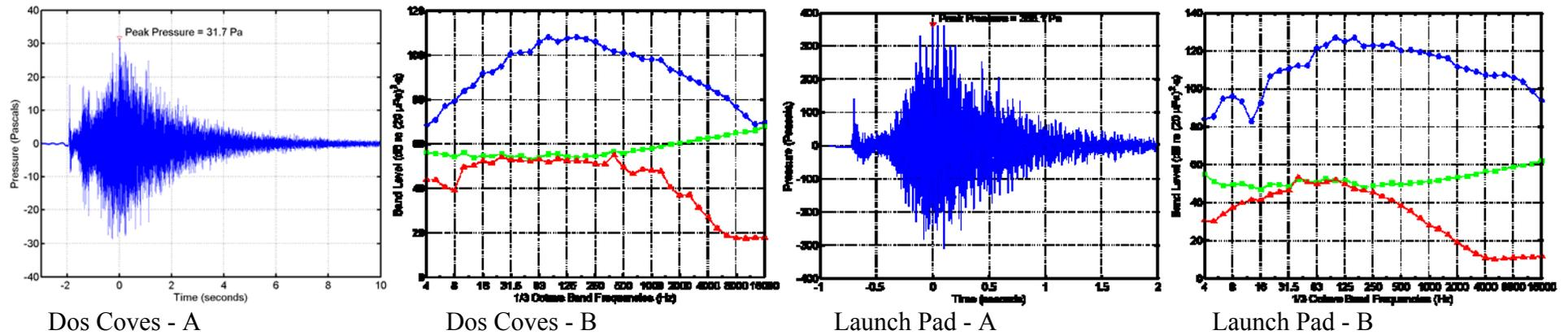
**FIGURE B-9. (A) Pressure waveform and (B) one-third octave band levels for a Terrier-Lynx flight at 02:33 on 28 March 2012.**
