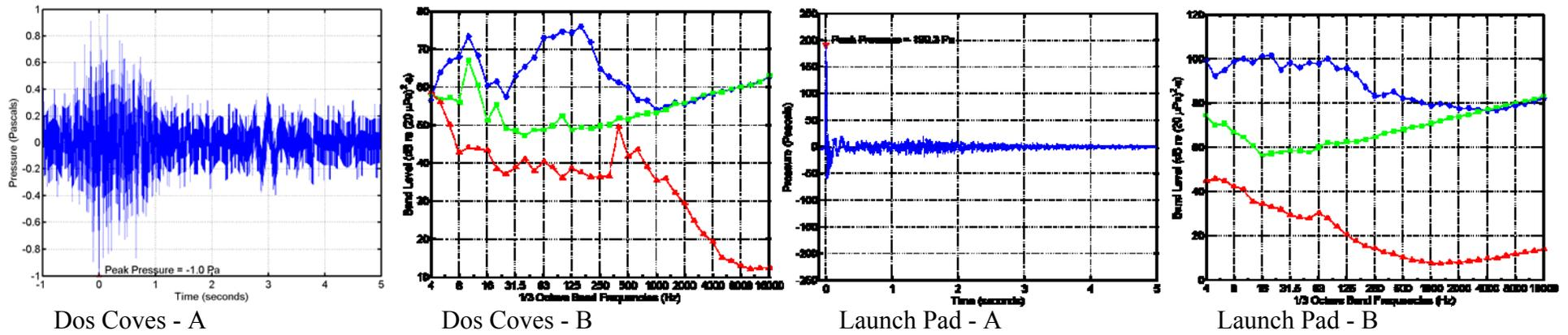
**FIGURE B-6. (A) Pressure waveform and (B) one-third octave band levels for a GQM flight at 12:45 on 7 December 2011.**
