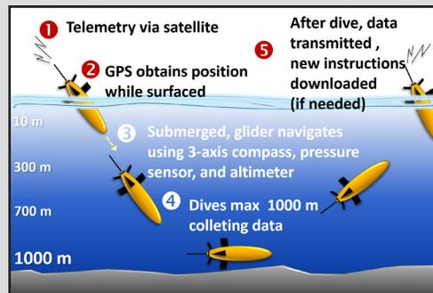
**Figure 5.** Dive sequence for the underwater Seaglider™.
