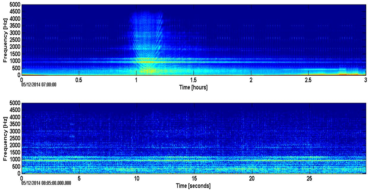
**Figure 14. Broadband ship noise in the LTSA (top) and spectrogram (bottom) at site CB.**
