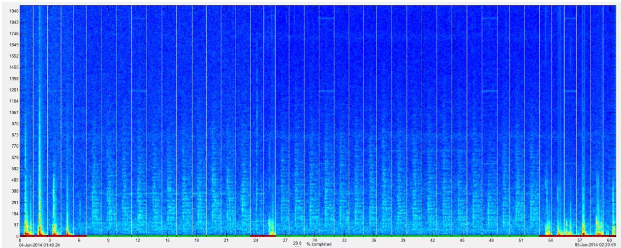
**Figure 17. Example of explosions from site PT in the analyst verification stage of the detector. Green in the bottom evaluation line indicates true and red indicates false detections.**
