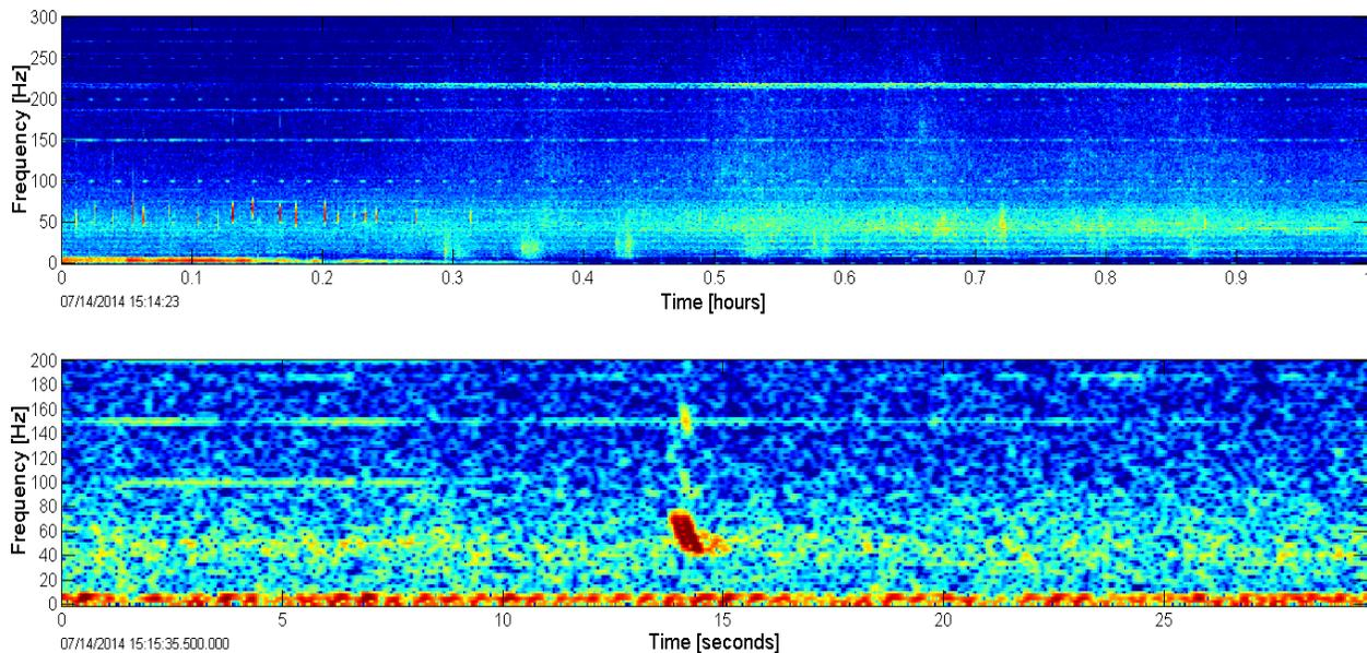
**Figure 6. Fin whale 40 Hz call in the LTSA (top) and spectrogram (bottom) at site CB.**
