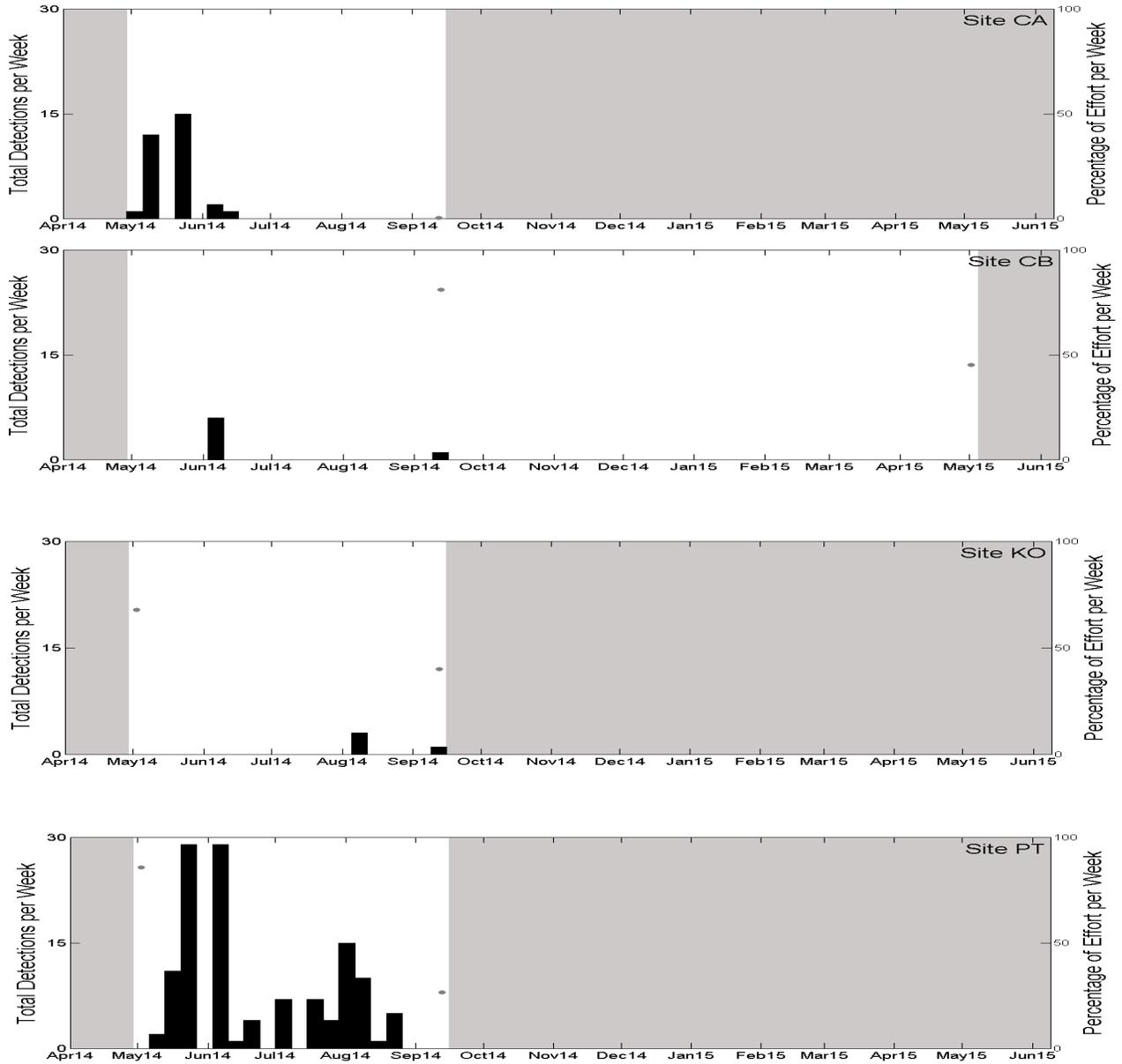
**Figure 45. Weekly detections of explosions between April 2014 and May 2015 at sites CA (top), CB (second from top), KO (second from bottom), and PT (bottom) were detected automatically using a matched filter detector. Effort markings are described in Figure 23.**
