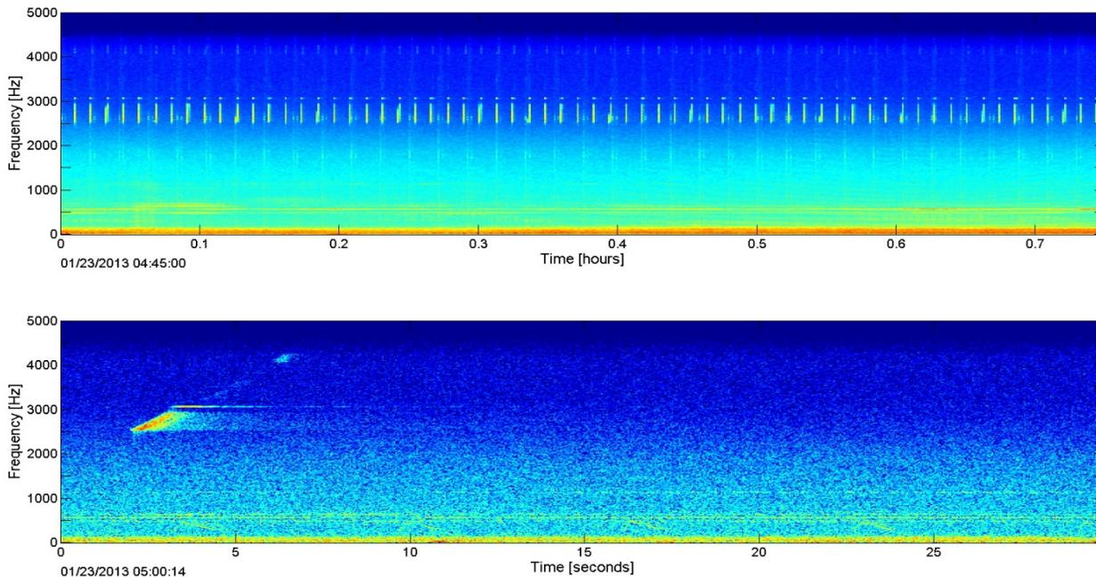
**Figure 15. Example of MFA sonar in the LTSA (top) and spectrogram (bottom) from a recording site off the coast of Washington.**
