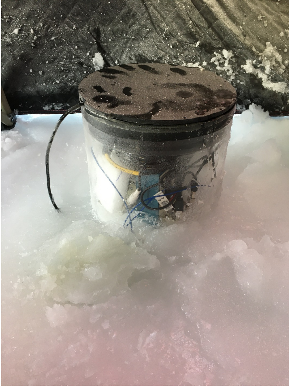
Figure 2 - Cryophone embedded in ice.
