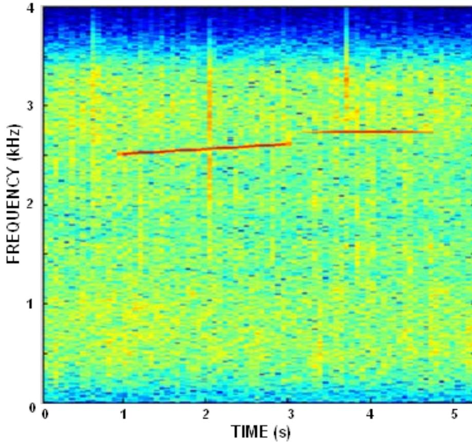
**Figure 5.** A spectrogram of a mid-frequency sonar ping at time between 1 and 3 seconds. The second shorter signal may be a reflection from the surface.
