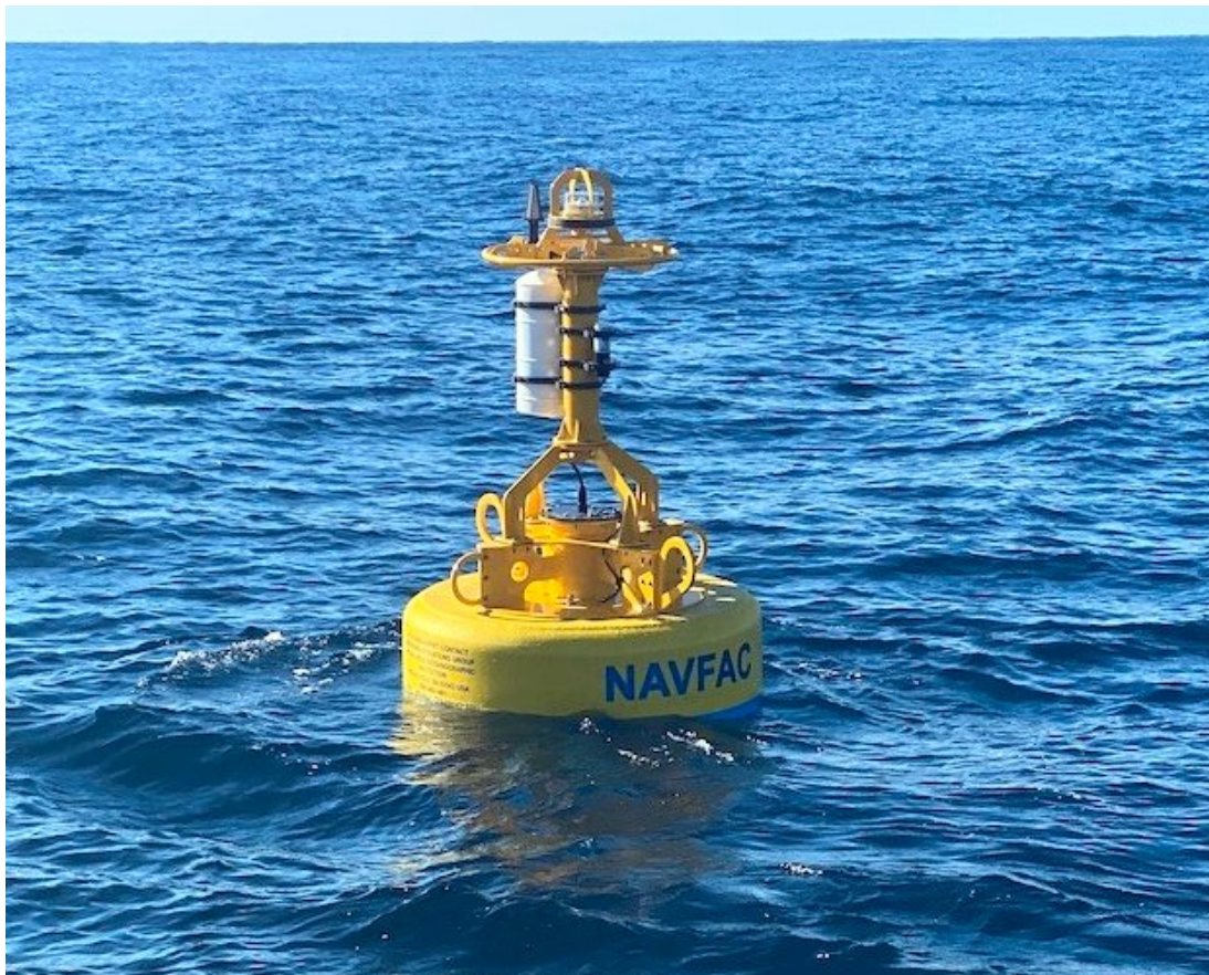
Figure 14. DMON buoy deployed off the coast of Cape Hatteras North Carolina.
