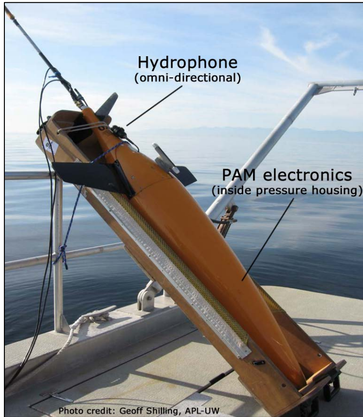
Figure 2: Passive-acoustic Seaglider. The Seaglider™ is a commercial off-the-shelf instrument sold by Kongsberg, Inc. (Lynwood, WA, USA). The PAM system was developed and incorporated into the Seaglider by APL-UW (Seattle, WA, USA).
