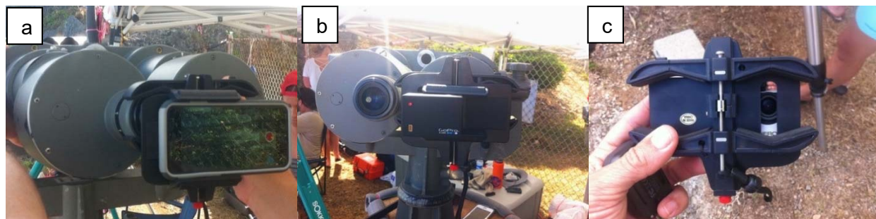
Figure 3. SnapZoom ocular mount for taking photos or video with an: iPhone (a) or GoPro (b and c) using the 25 \times magnification from the Big Eyes.
