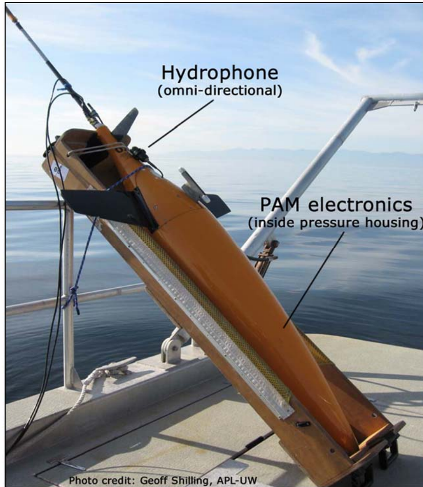
Figure 2: Passive-acoustic Seaglider. The Seaglider™ is a commercial off-the-shelf instrument sold by Kongsberg, Inc. (Lynwood, Washington, USA). The PAM system was developed and incorporated into the Seaglider by APL-UW (Seattle, Washington, USA).
