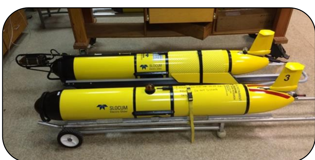
Fig. 2. Autonomous platforms: Gliders from NAVO (top) and WHOI (bottom) prepared for deployment. Note that the DMON hardware is integrated in the WHOI glider, while the NAVO glider uses an older DMON deployment strategy.
