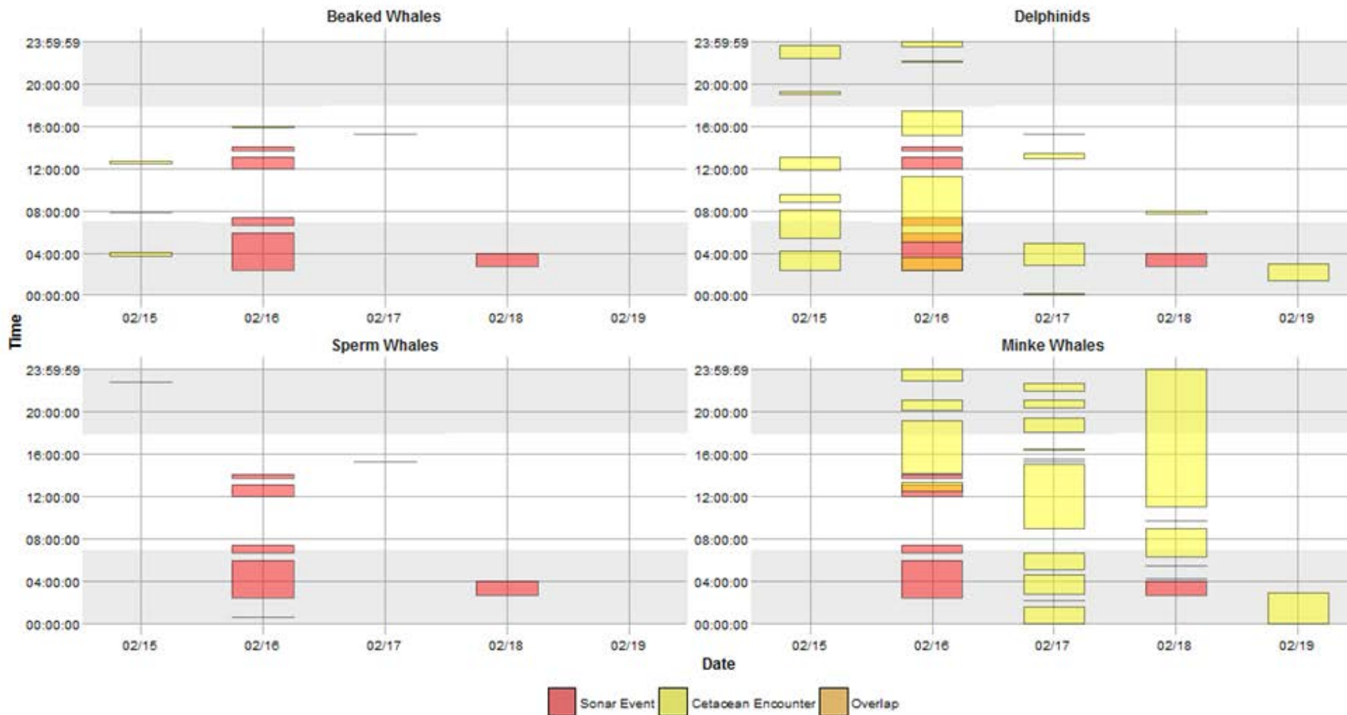
Figure 91. Sonar events (pink) and vocalization events (yellow) by species or species group for the Onslow Bay 1 (USWTR05A) HARP deployed in Onslow Bay, North Carolina. Time of day is plotted on the y-axis, date is plotted on the x-axis, and shading represents periods of light and darkness.
