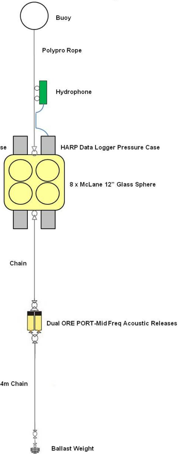
Figure 2. Schematic diagram showing details of the Norfolk Canyon 01A HARP. Note that diagram is not drawn to scale.
