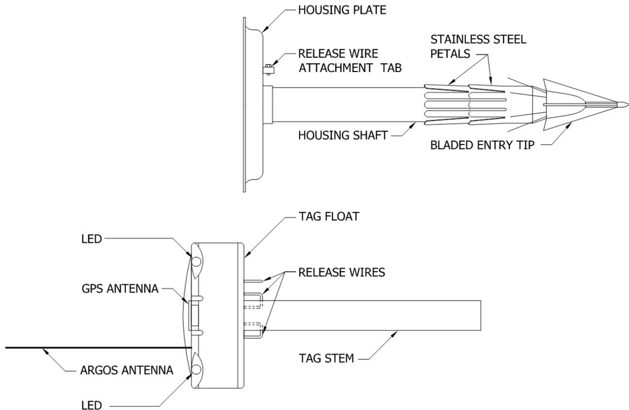
**Figure 2. Schematic of the design of the Advanced Dive Behavior (ADB) tag used in this project. Taken from Mate et al. (in prep).**
