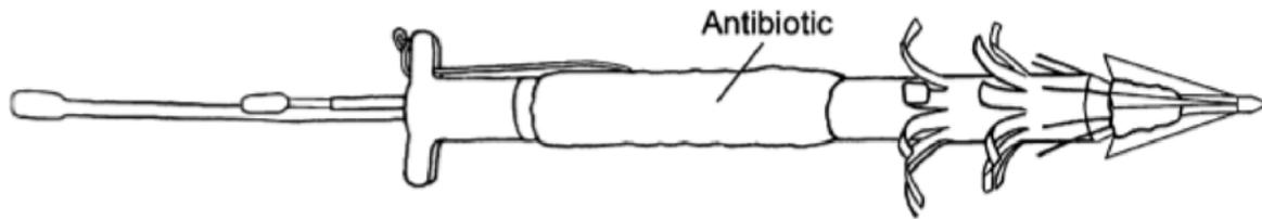
**Figure 1. Schematic of the design of the location-only tag, such as the SPOT5 used in this project, showing the main body, the antenna/saltwater conductivity switch endcap, the penetrating tip, the anchoring system, and the antibiotic coating. Taken from Mate et al. (2007).**
