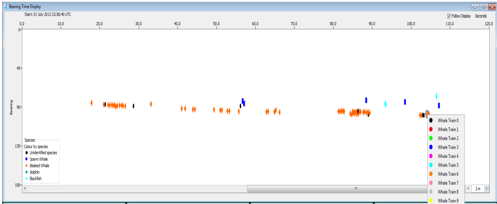
Figure A-1. PAMGuard click detector display showing the bearing (y-axis) versus time (x-axis) display with detected clicks represented as filled shapes with the color indicating automatic classification of species or species groups. Using the 'semi-automated method,' selected clicks can be manually assigned by the user to a 'whale train,' which is then sent to ROCCA for measurement. In contrast, in the 'automated method' all clicks colored as the species of interest (e.g., beaked whale (orange) would be sent to ROCCA for measurement).
