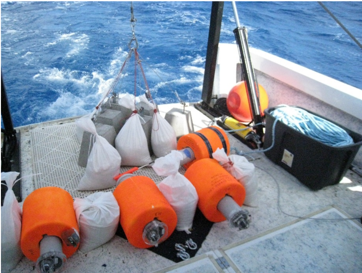
Figure 3. Bottom-moored EAR2 array showing four EAR2s, an acoustic release, 300 meters of line, and anchor (concrete blocks and sand bags).
