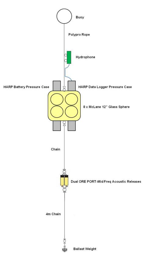
Figure 3. Schematic diagram showing details of a compact small mooring HARP. Note that diagram is
