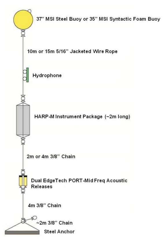
Figure 1. Schematic diagram showing details of a large mooring HARP. Note that diagram is not
