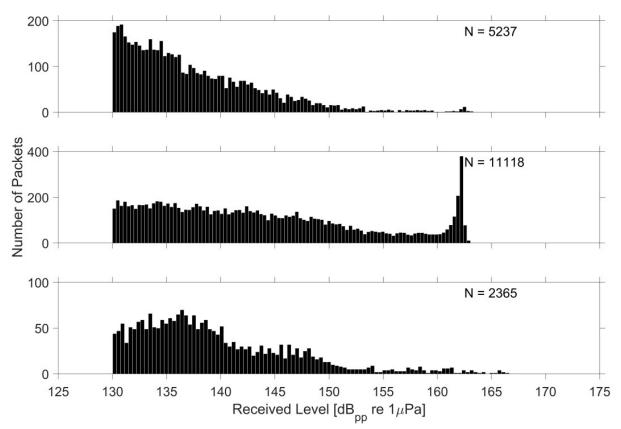
Figure 20. MFA sonar packet peak-to-peak received level distributions for sites H (top), N (middle), and P (bottom). The total number of packets detected at each site is given in the upper right corner of each panel. Instrument clipping levels are reached at 161-163 dB $_{pp}$  re 1  $\mu$ Pa (range due to signal filtering). Note the vertical axes are at different scales.
