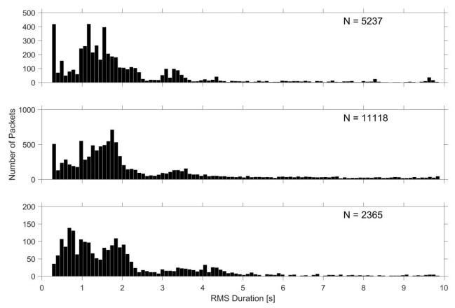
Figure 21. MFA sonar packet RMS duration distributions for sites H (top), N (middle), and P (bottom). The total number of packets detected is given in the top right corner of each panel. Note the vertical axes are at different scales.
