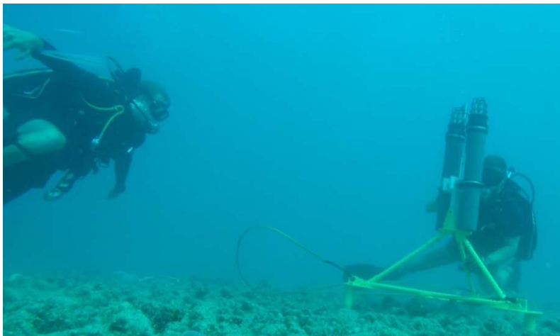
Figure 4. Photograph of the autonomous recording system (see Figure 1 green triangle, dual system) deployed at range 1500 from the UNDET site showing U.S. Navy divers from CO 1-8 making final adjustments on the deployment.
