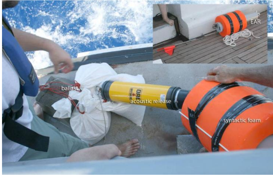
Figure 10. Components of the EAR device. Pictured are ballast (cement and sand bag), acoustic release, syntactic foam float with signal flag, and EAR acoustic recording device.
