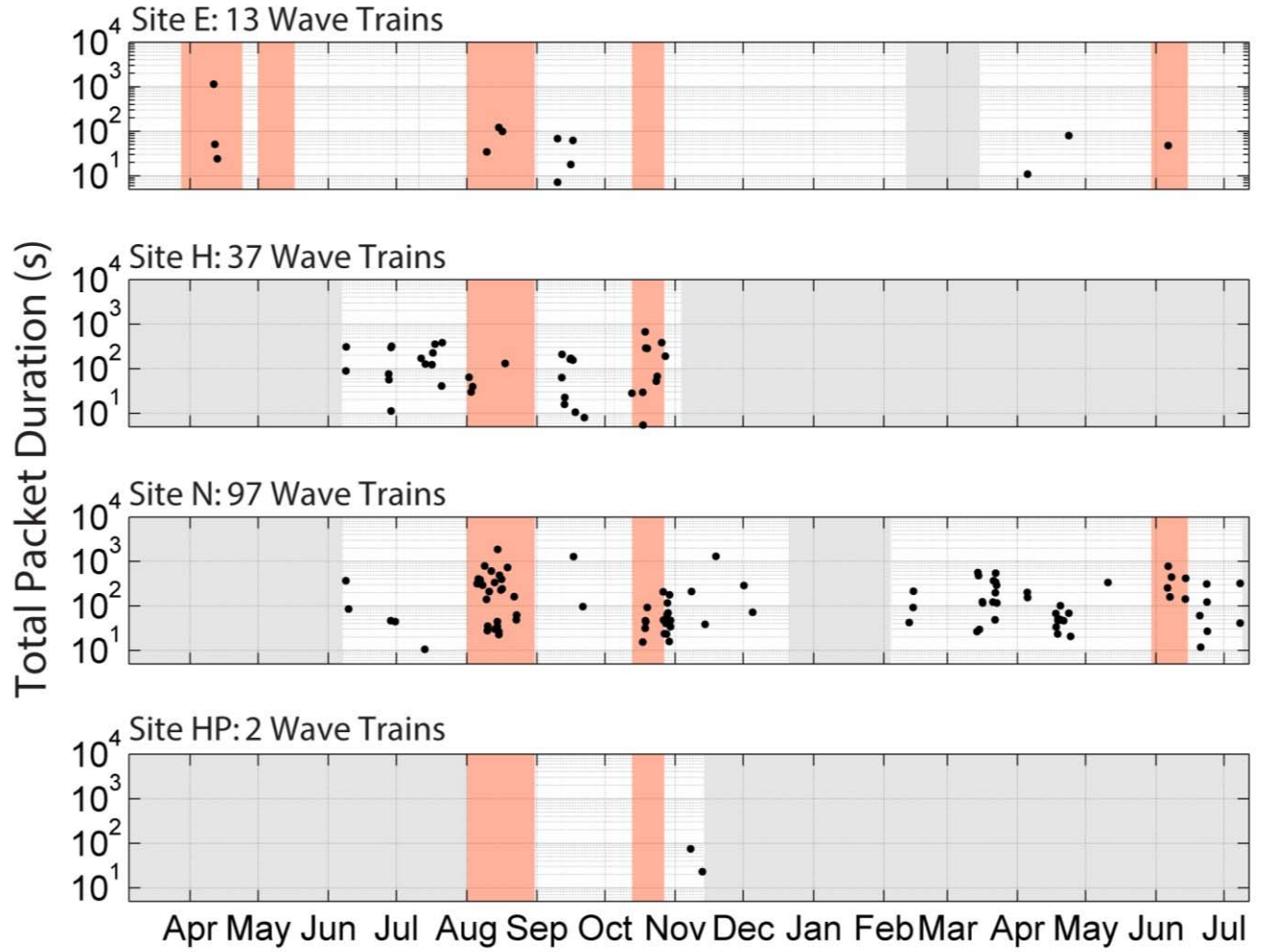
Figure 30. Total packet duration for each wave train at sites E, H, N, and HP. Note the vertical axes are logarithmic base-10.
