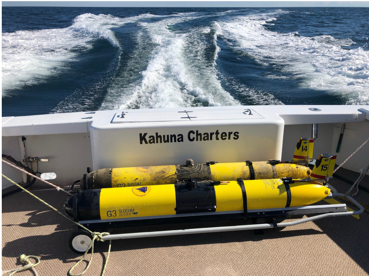
Figure 4. Gliders we14 and we15 after recovery on March 18, 2019. Note difference in biofouling – we14 was deployed south of Cape Hatteras and has much more biofouling than we15, which was deployed north of Cape Hatteras. Also, note the protective cage over the hydrophone on we15, while the cage on we14 was removed when it was intercepted to clean out the nose cone on February 1.
