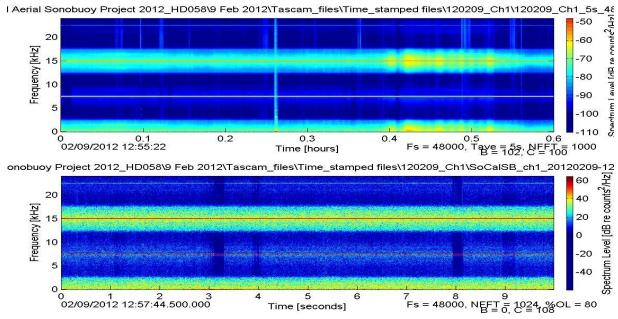
9 10 Figure 1. Example of an LTSA (top panel) and spectrogram (bottom panel) with a good DF signal.
