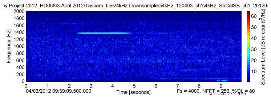
Figure 14. Spectrogram of a mid-frequency sonar signal centered at 1.375 kHz recorded from a sonobuoy on 3 April.
