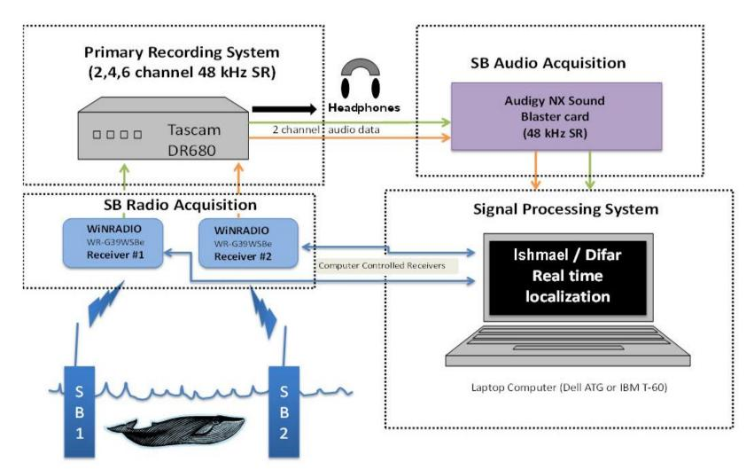
*Figure 1.* Block diagram of sonobuoy signal acquisition, recording, and processing system.
