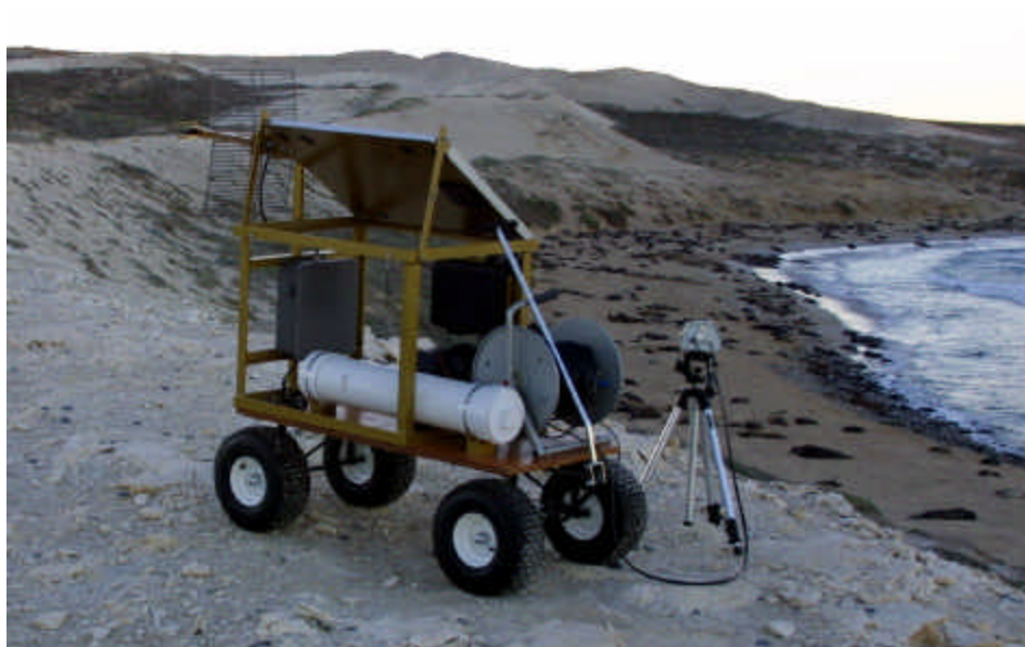
FIGURE 3.2. View of a wagoncam, which unlike other portable video cameras, can transmit its signal back to a centralized location where it is recorded. (Photograph by U.S. Navy)
