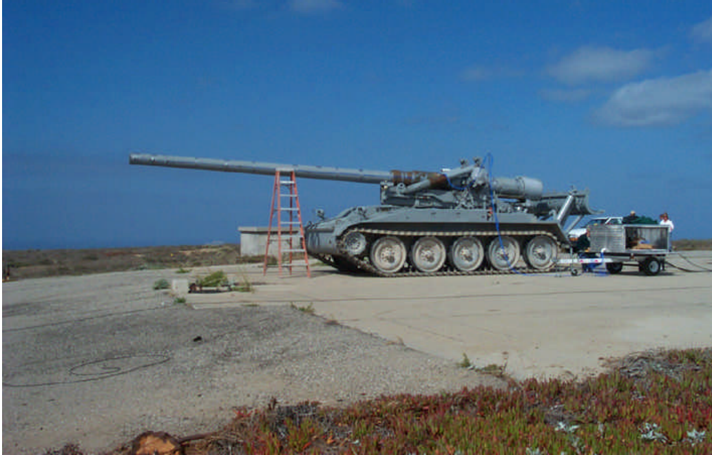
FIGURE 1.6. View of the Advanced Gun Projectile Test System at the Alpha Complex on San Nicolas Island (photograph by U.S. Navy).
