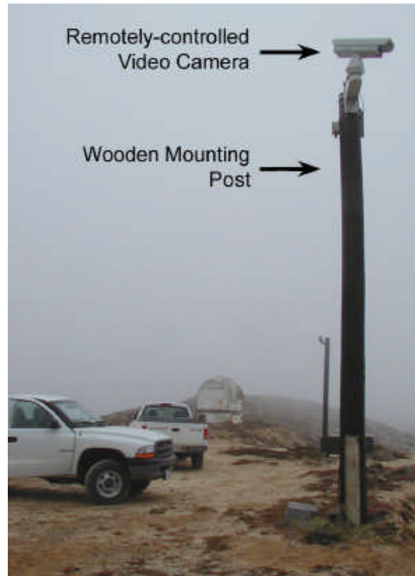
FIGURE 3.1. View of permanent fixed video camera atop a wooden post at 809 Camera. This camera can be remotely zoomed, tilted, and panned. Digital data from this camera were sent back to a distant blockhouse where they were recorded on large-format digital videotape. An ATAR was deployed near the base of the camera pole during most launches. (Photograph by J. Lawson, LGL.)
