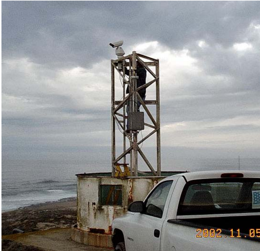
FIGURE 3.1. View of the permanent fixed video camera at Building 809. This camera can be remotely zoomed, tilted, and panned, but was non-operational during the present monitoring period. (Photograph by U.S. Navy)
