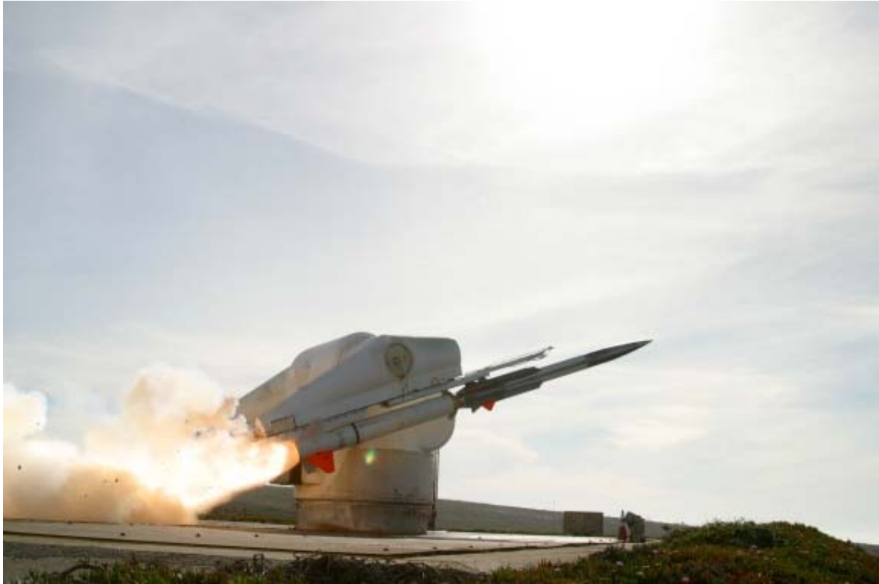
FIGURE 1.3. View of the GQM-163A SSST with booster and launcher at the Alpha Launch Complex on San Nicolas Island (photograph by U.S. Navy).
