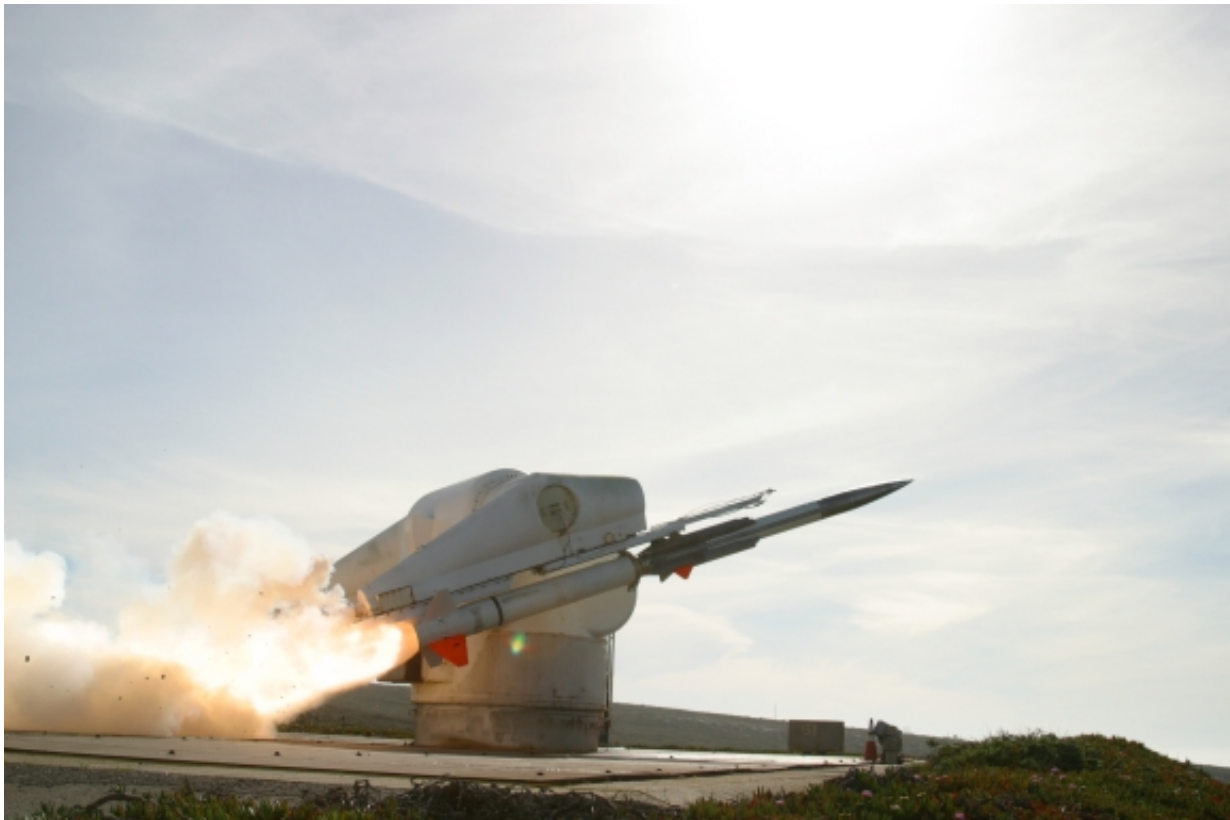
FIGURE 1.5. View of the GQM-163A SSST with booster and launcher at the Alpha Launch Complex on SNI (photograph by U.S. Navy).
