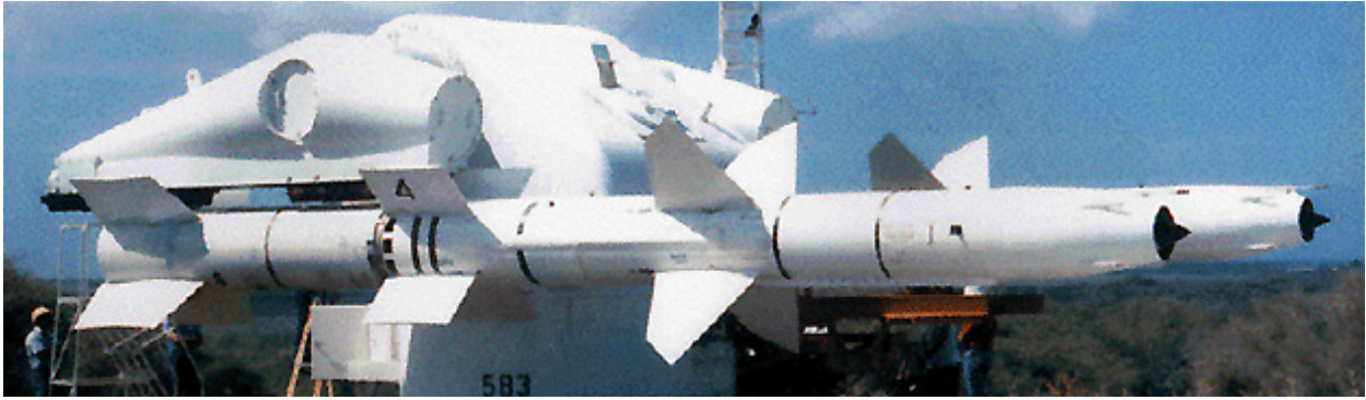
FIGURE 1.4. View of two Vandals mounted on the launch pad at the Alpha Complex on SNI; solid rocket booster is visible at rear of closer Vandal (photograph by U.S. Navy).
