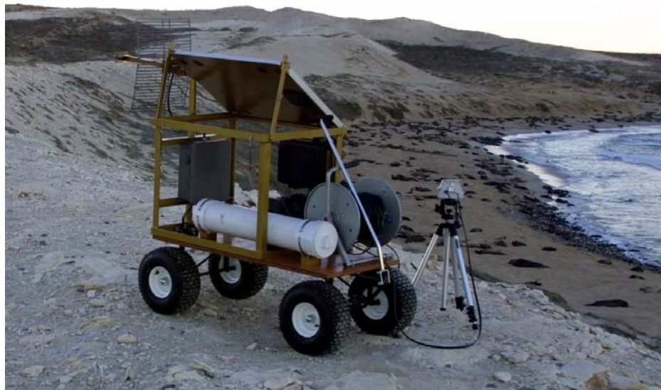
FIGURE 3.3. View of a wagoncam, which unlike other portable video cameras, can transmit its signal back to a centralized location where it is recorded. (Photograph by U.S. Navy)
