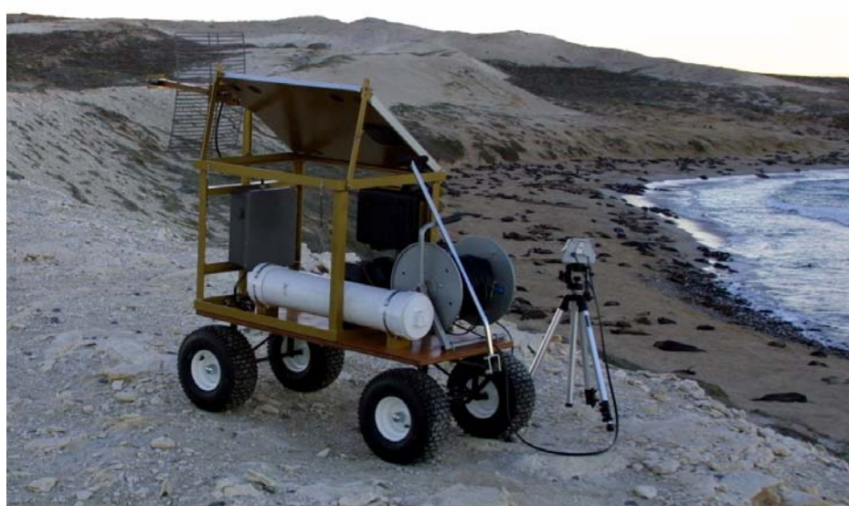
FIGURE 3.2. View of a wagoncam. Unlike other portable video cameras, a wagoncam can transmit its signal back to a centralized location where it is recorded. (Photograph by U.S. Navy).
