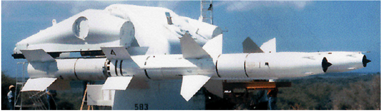
FIGURE 1.4. Two Vandals mounted on the launch pad at the Alpha Complex on SNI; solid rocket booster is visible at rear of closer Vandal (photograph by U.S. Navy).
