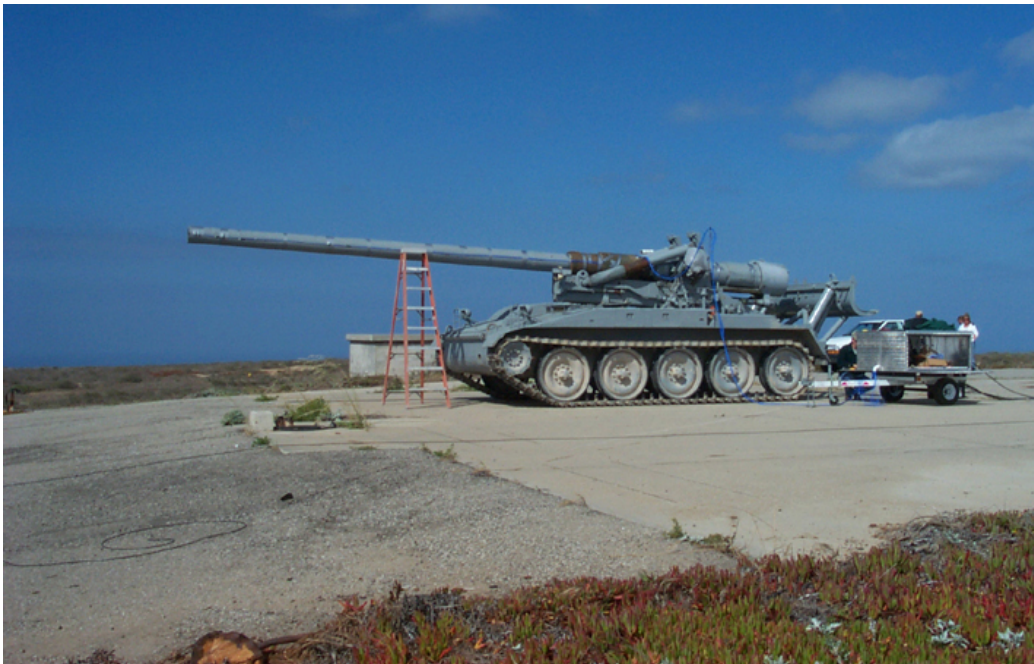
FIGURE 1.11. Howitzer used as AGS launcher at the Alpha Complex on SNI (photograph by U.S. Navy).
