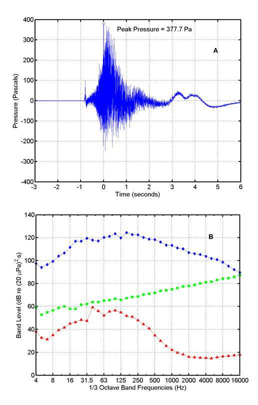
FIGURE B-9. (A) Pressure waveform and (B) one-third octave band levels for a Terrier-Black Brant flight at 20:50 on 10 August 2009 recorded near the Launcher. In (B),  $\Diamond =$  missile sound energy;  $\Box =$  instrumentation noise energy;  $\Delta =$  ambient noise power. Band frequencies in Hertz (Hz).
