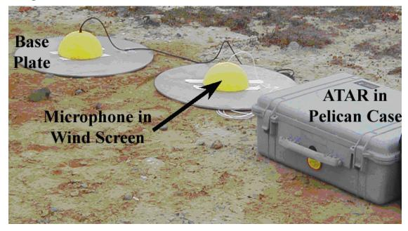
FIGURE 2.3. Typical field installation of an ATAR at SNI, California (photograph by J. Lawson, LGL).
