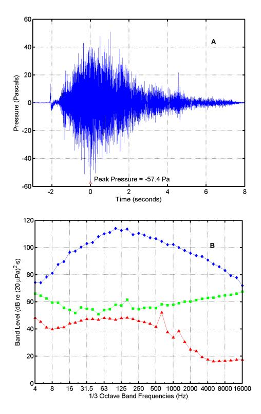
FIGURE B-6. (A) Pressure waveform and (B) one-third octave band levels for a Terrier-Black Brant flight at 20:50 on 10 August 2009 recorded at Dos Coves South. In (B),  $\Diamond$  = missile sound energy;  $\Box$  = instrumentation noise energy;  $\Delta$  = ambient noise power. Band frequencies in Hertz (Hz).
