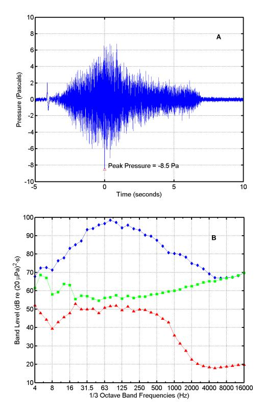
FIGURE B-2. (A) Pressure waveform and (B) one-third octave band levels for a Terrier-Lynx flight at 22:16 on 6 June 2009 recorded at Redeye Beach. In (B),  $\Diamond$  = missile sound energy;  $\Box$  = instrumentation noise energy;  $\Delta$  = ambient noise power. Band frequencies in Hertz (Hz).
