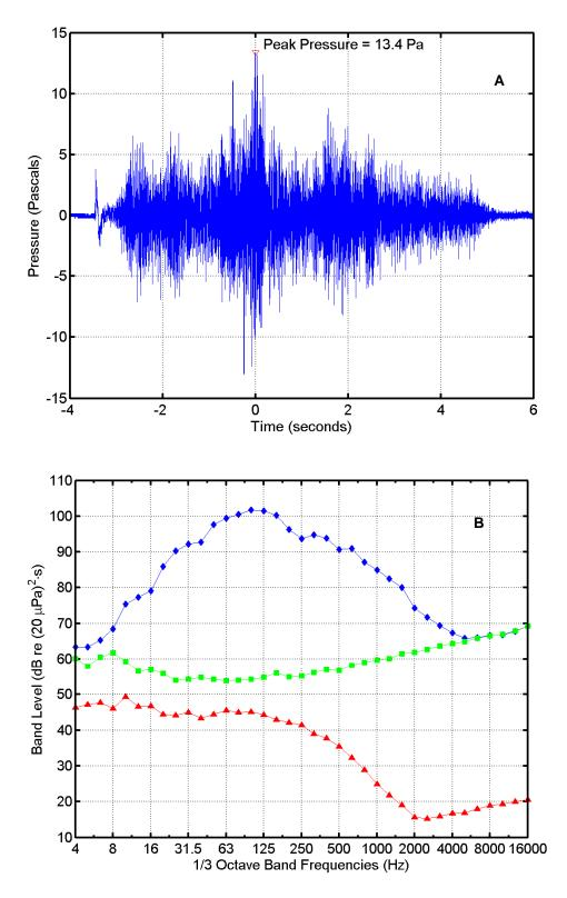
FIGURE B-11. (A) Pressure waveform and (B) one-third octave band levels for a Terrier-Black Brant flight at 02:46 on 3 May 2010 recorded at N165. In (B),  $\Diamond$  = missile sound energy;  $\Box$  = instrumentation noise energy;  $\Delta$  = ambient noise power. Band frequencies in Hertz (Hz).
