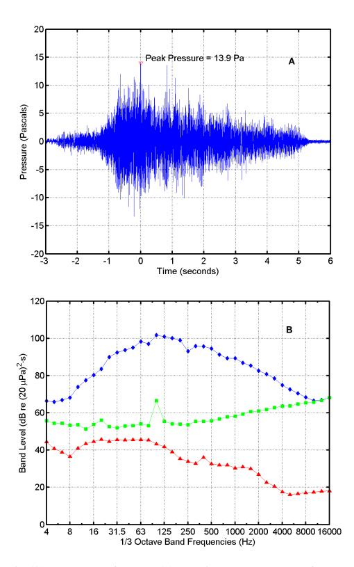
FIGURE B-8. (A) Pressure waveform and (B) one-third octave band levels for a Terrier-Black Brant flight at 20:50 on 10 August 2009 recorded at The "Y". In (B),  $\Diamond$  = missile sound energy;  $\Box$  = instrumentation noise energy;  $\Delta$  = ambient noise power. Band frequencies in Hertz (Hz).
