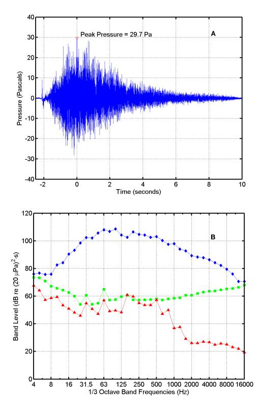
FIGURE B-4. (A) Pressure waveform and (B) one-third octave band levels for a Terrier-Lynx flight at 22:31 on 13 June 2009 recorded at Bachelor Beach North. In (B),  $\Diamond$  = missile sound energy;  $\Box$  = instrumentation noise energy;  $\Delta$  = ambient noise power. Band frequencies in Hertz (Hz).
