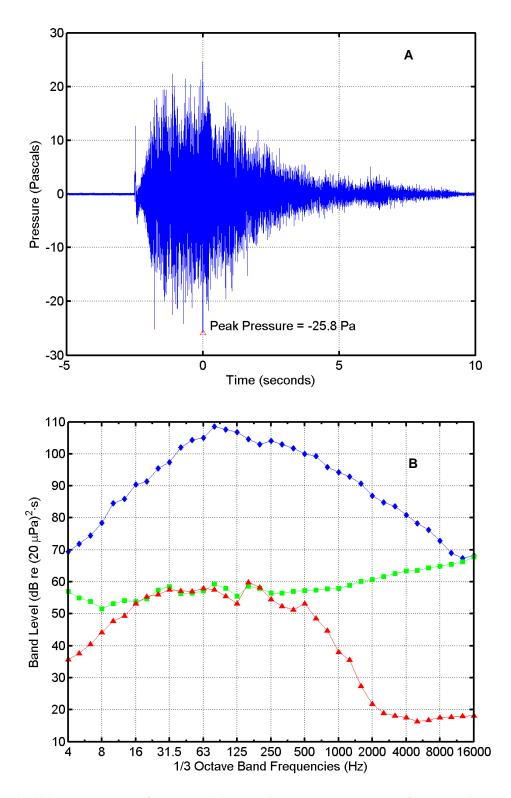
FIGURE B-1. (A) Pressure waveform and (B) one-third octave band levels for a Terrier-Lynx flight at 22:16 on 6 June 2009 recorded at Bachelor Beach North. In (B),  $\Diamond =$  missile sound energy;  $\Box =$  instrumentation noise energy;  $\Delta =$  ambient noise power. Band frequencies in Hertz (Hz).
