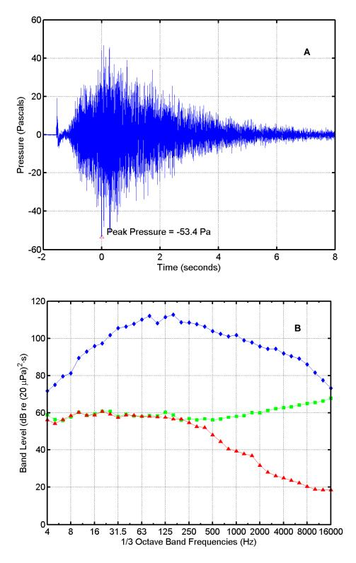
FIGURE B-10. (A) Pressure waveform and (B) one-third octave band levels for a Terrier-Black Brant flight at 02:46 on 3 May 2010 recorded at Dos Coves South. In (B),  $\Diamond$  = missile sound energy;  $\Box$  = instrumentation noise energy;  $\Delta$  = ambient noise power. Band frequencies in Hertz (Hz).
