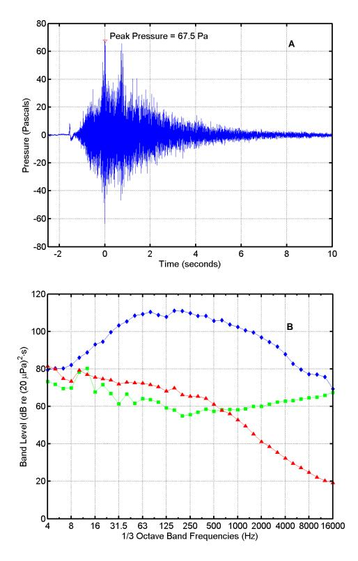
FIGURE B-3. (A) Pressure waveform and (B) one-third octave band levels for a Terrier-Lynx flight at 22:31 on 13 June 2009 recorded at Dos Coves South. In (B),  $\Diamond$  = missile sound energy;  $\Box$  = instrumentation noise energy;  $\Delta$  = ambient noise power. Band frequencies in Hertz (Hz).
