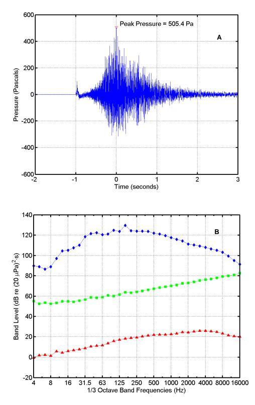
FIGURE B-12. (A) Pressure waveform and (B) one-third octave band levels for a Terrier-Black Brant flight at 02:46 on 3 May 2010 recorded near the Launcher. In (B),  $\Diamond =$  missile sound energy;  $\Box =$  instrumentation noise energy;  $\Delta =$  ambient noise power. Band frequencies in Hertz (Hz).
