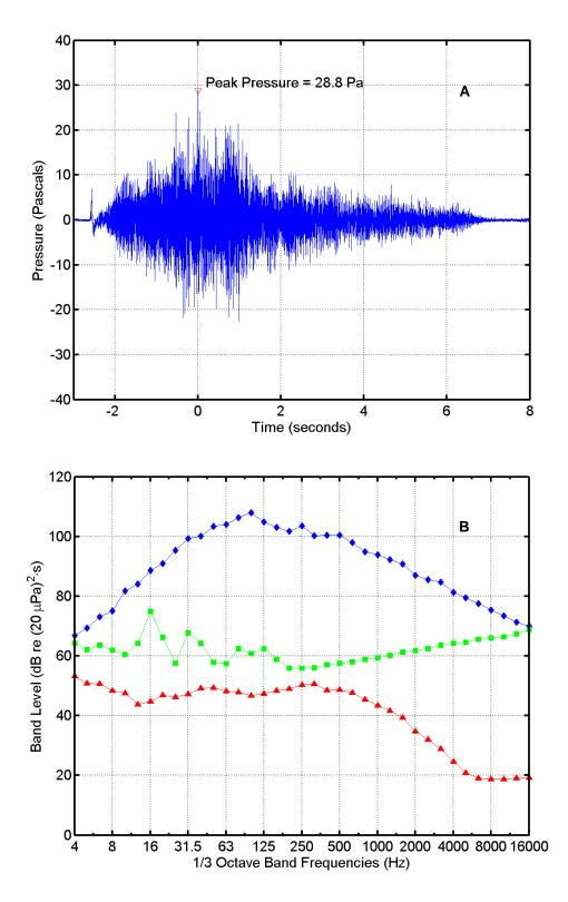
FIGURE B-7. (A) Pressure waveform and (B) one-third octave band levels for a Terrier-Black Brant flight at 20:50 on 10 August 2009 recorded at Bachelor Beach South. In (B),  $\Diamond =$  missile sound energy;  $\Box =$  instrumentation noise energy;  $\Delta =$  ambient noise power. Band frequencies in Hertz (Hz).
