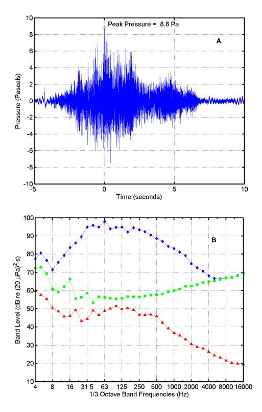
FIGURE B-5. (A) Pressure waveform and (B) one-third octave band levels for a Terrier-Lynx flight at 22:31 on 13 June 2009 recorded at Redeye Beach. In (B),  $\Diamond =$  missile sound energy;  $\Box =$  instrumentation noise energy;  $\Delta =$  ambient noise power. Band frequencies in Hertz (Hz).
