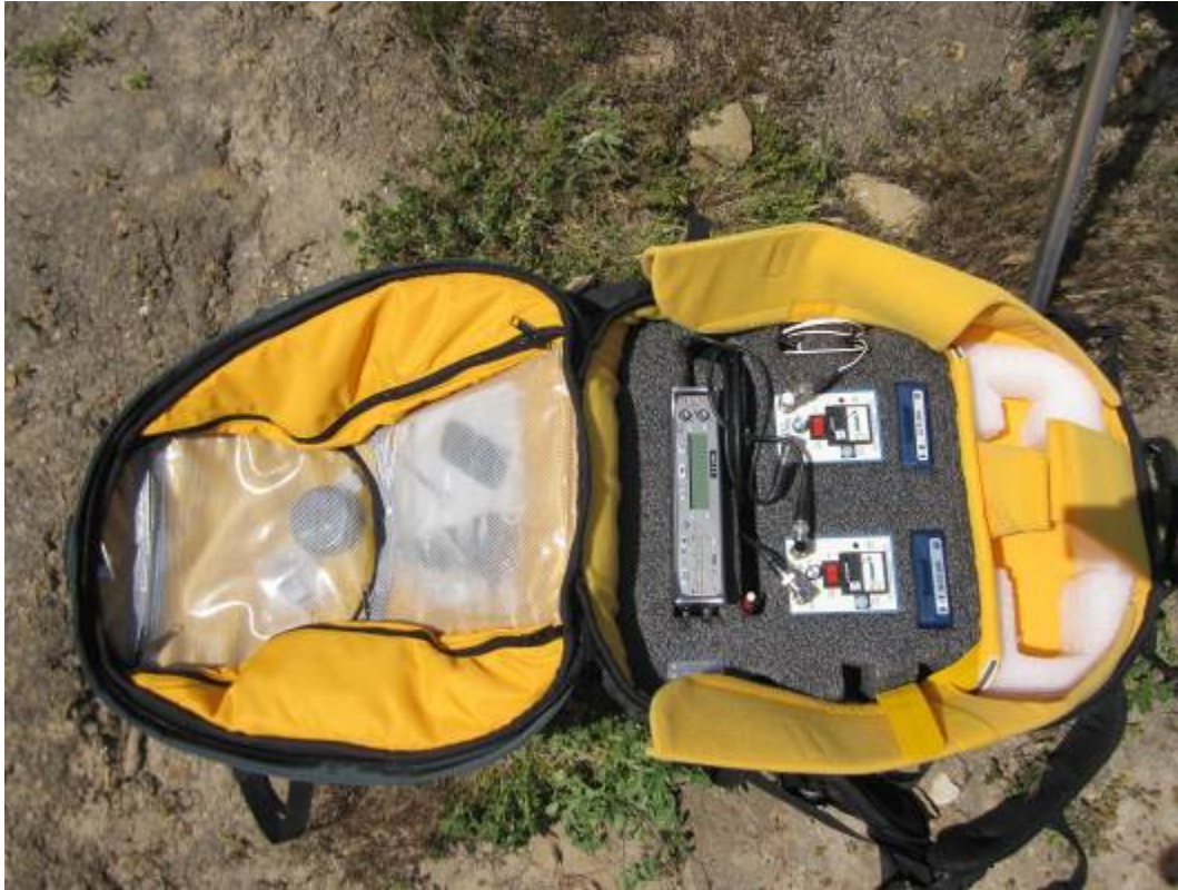
FIGURE 2.2. Photo of ATAR components in waterproof backpack (photograph by J. Ugoretz, U.S. Navy).
