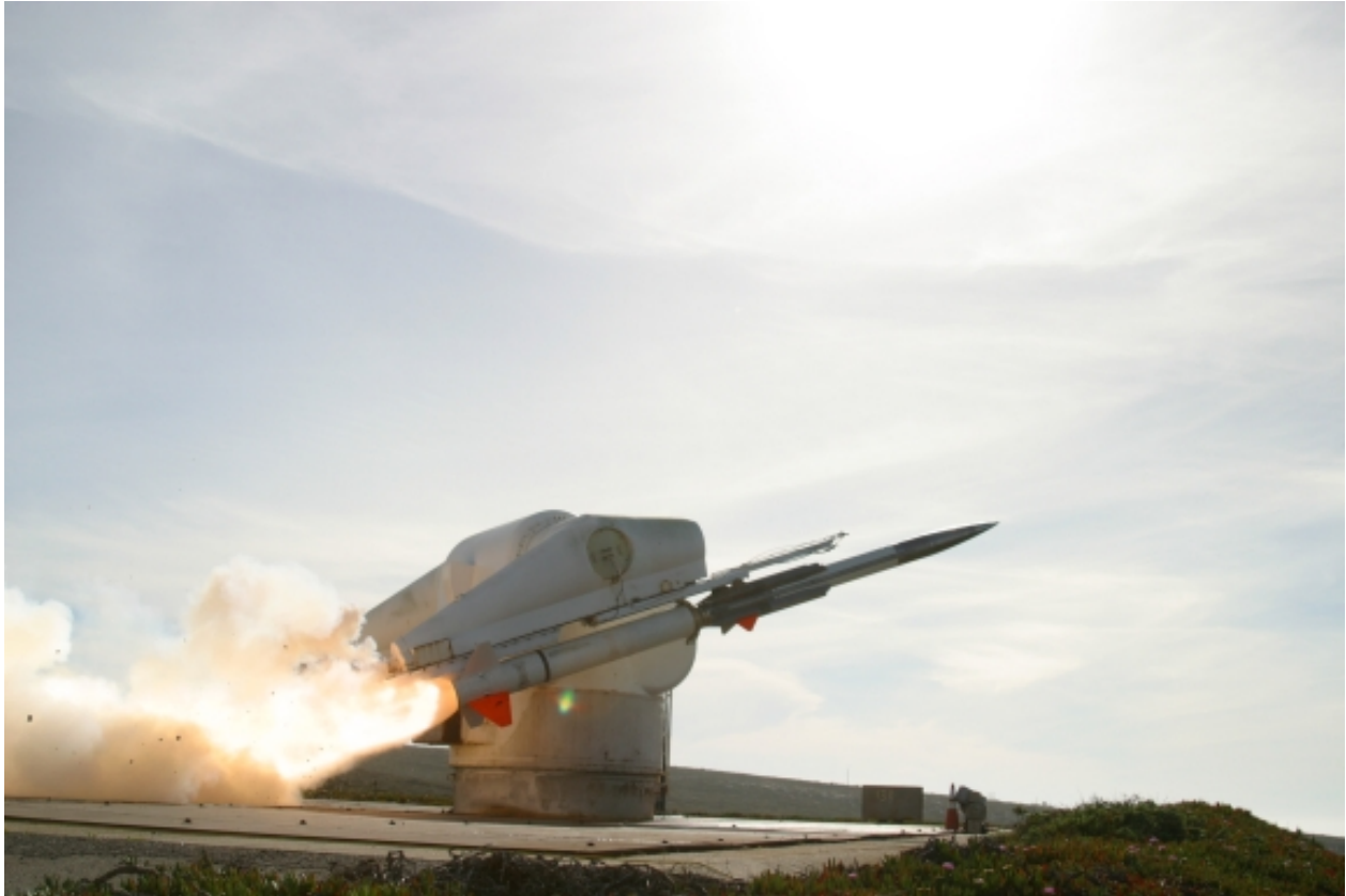
FIGURE 1.3. GQM-163A SSST with booster and launcher at the Alpha Launch Complex on SNI (photograph by U.S. Navy).
