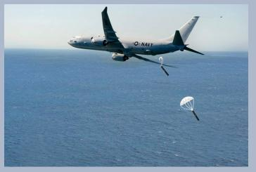
DICASS sonobuoy Directional Command-Activated Sonobuoy System
