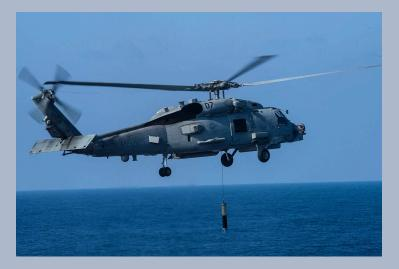
Helicopter-dipping AN/AQS-22, 4.1 kHz, source level 217 dB
