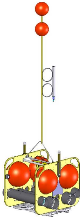
Figure 6. Standard seafloor-mounted High-frequency Acoustic Recording Package configuration.
