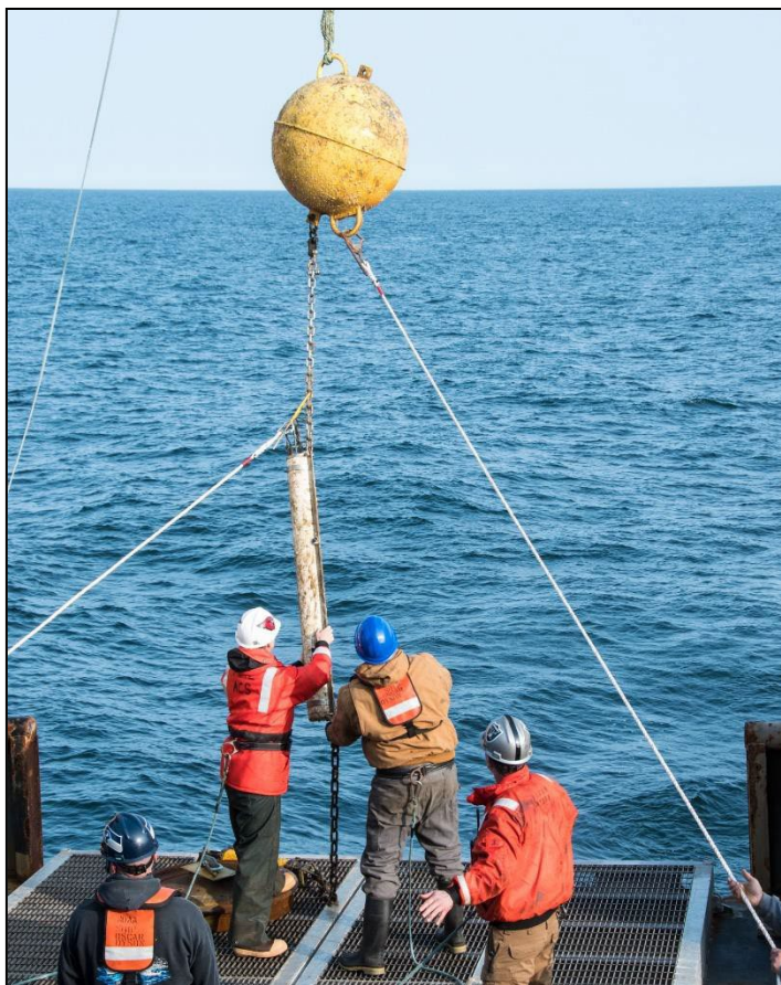
Figure 7. Long-term bottom mounted passive acoustic recorder retrieval on the NOAA ship Oscar Dyson.
