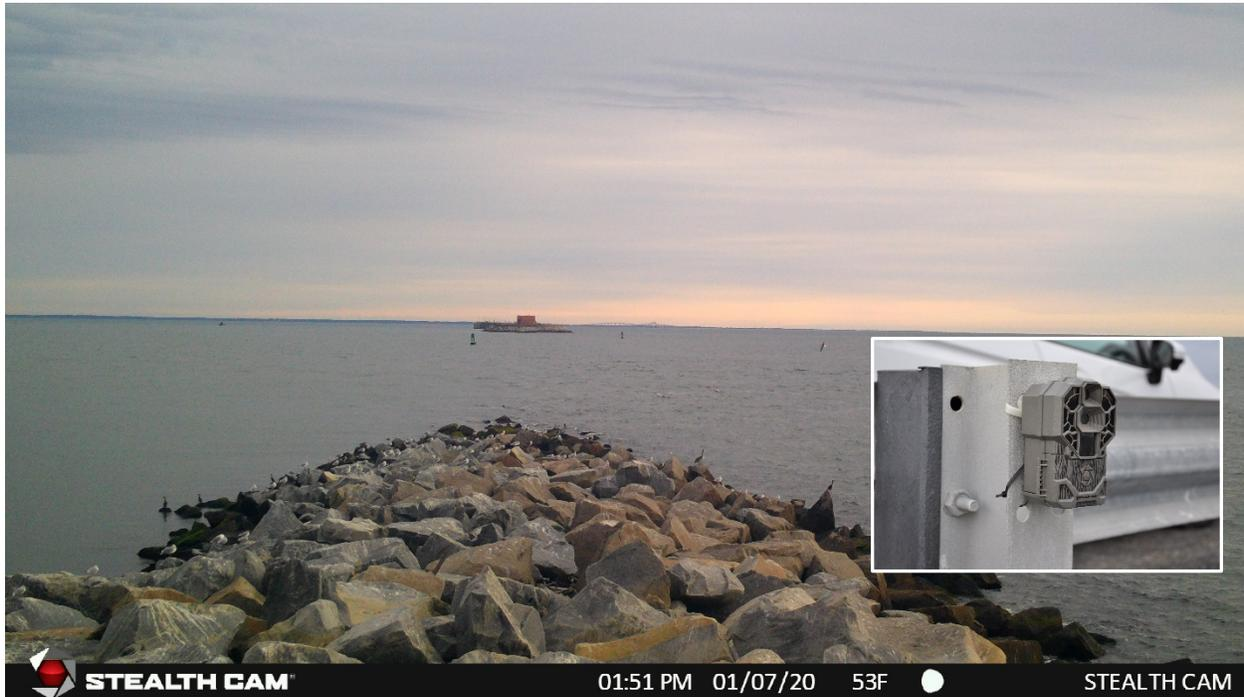
Figure 2-5. Camera view of CBBT3 and image of camera installed on the guardrail (inset).
