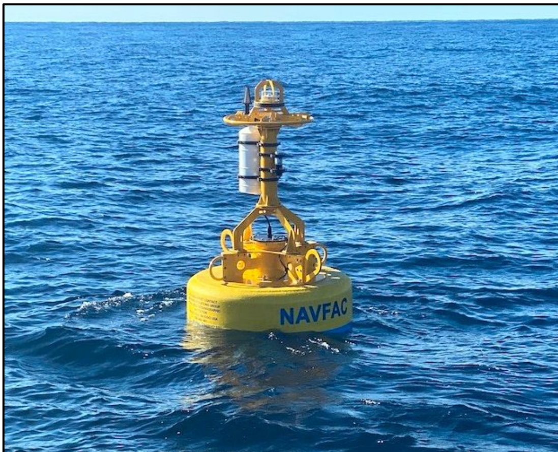
Figure 24. DMON buoy deployed off the coast of Cape Hatteras, North Carolina.
