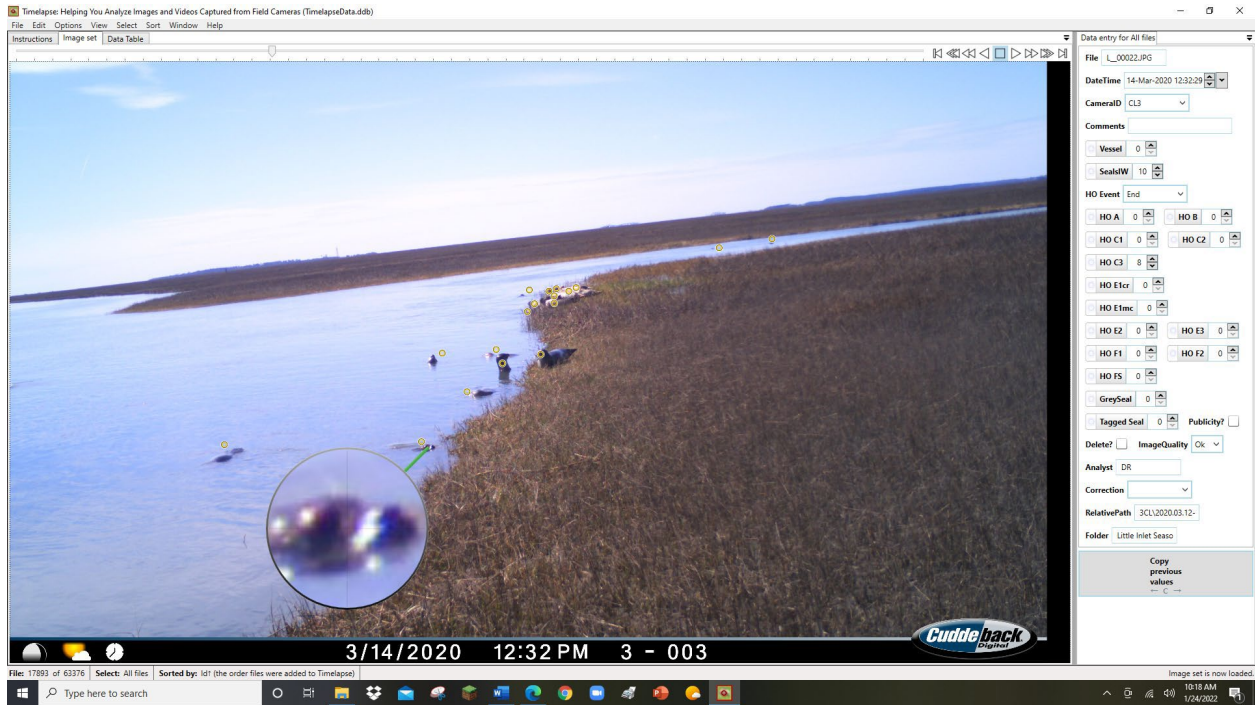
Figure 16. Screenshot of Timelapse Image Analysis workspace. Counted seals are marked by yellow circles, the magnifier feature is shown near the front of the image and the customizable data template at the right.
