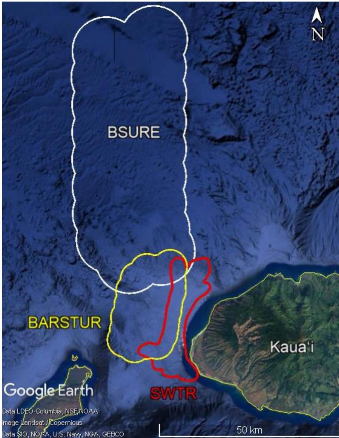
**Figure 1.** The PMRF hydrophone system showing range systems: Shallow Water Training Range (SWTR), the Barking Sands Tactical Underwater Range (BARSTUR), and Barking Sands Underwater Range Expansion (BSURE).
