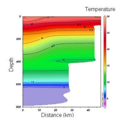
Figure 30: Temperature profiles at depth within a Gulf Stream frontal eddy produced from ecasts. Domed temperature contours at depth indicate the presence of the eddy cold core, while blank areas indicate bottom topography.
