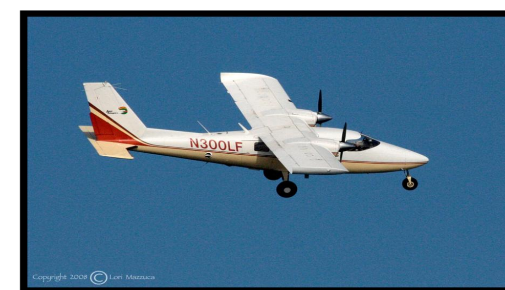
Partenavia P68-C; twin-engine, fixed-wing aircraft used as primary platform for aerial surveys flown at 800-1000 ft. altitude & 100 kt. Focal follows at 1200-1500 ft. altitude & 0.5-1 km radial distance.
